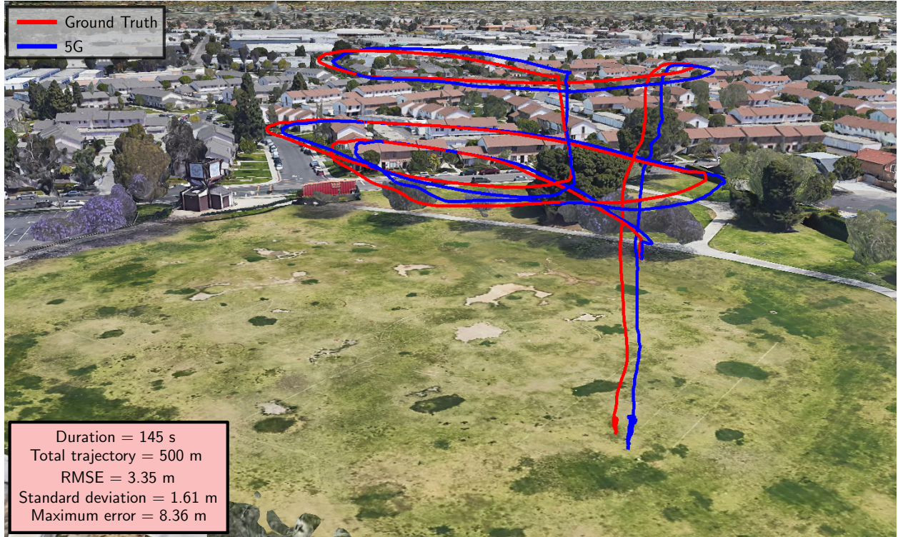
Figure 5.45: The 5G navigation solution exhibited a position RMSE of 3.35 m versus the ground-truth reference navigation solution. Image: Google Earth.
