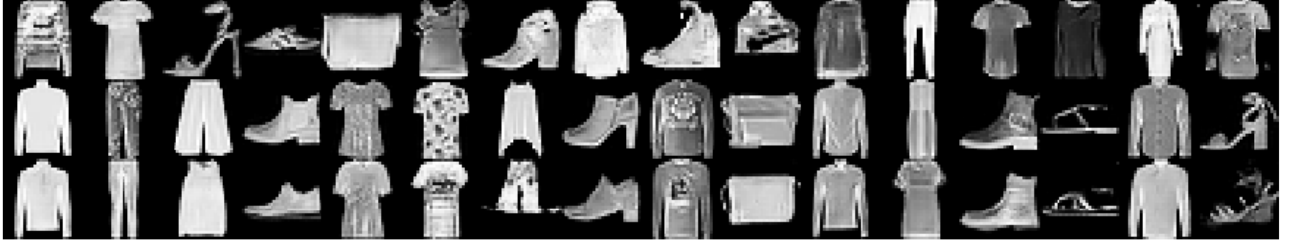
Figure C.5: BiGAN training results for Fashion-MNIST dataset, including generated samples G(z) (upper row), real data x (middle row), and corresponding reconstructions G(E(x)) (bottom row).
