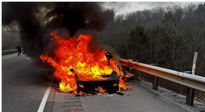
Figure 8.2 Tesla Model S e-vehicle in the midst of an unrolled lithium-ion battery fire [12].
