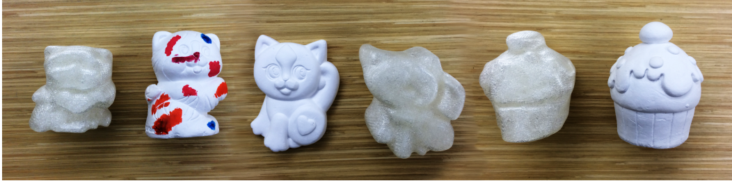
Figure 3.13: 3D Printing. We 3D printed the standing cat, flat cat, and cupcake examples. The printed examples showcase the capability of using passive camera systems with a single exposure to capture shape for 3D printing. Note that we scaled the printed figurines to fit in a 50mm cube with 0.2mm precision.
