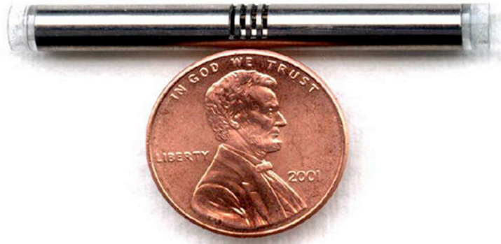
Figure 18. Implanted device fitted with nanopore membranes. (Top) Drawing illustrating key features of the device. The dashed arrows represents a possible diffusion path of a drug molecular held within the device reservoir. (Bottom) Photograph of prototype implant device illustrating its size in relation to a U.S. 1 cent piece. Reprinted with permission. 98
