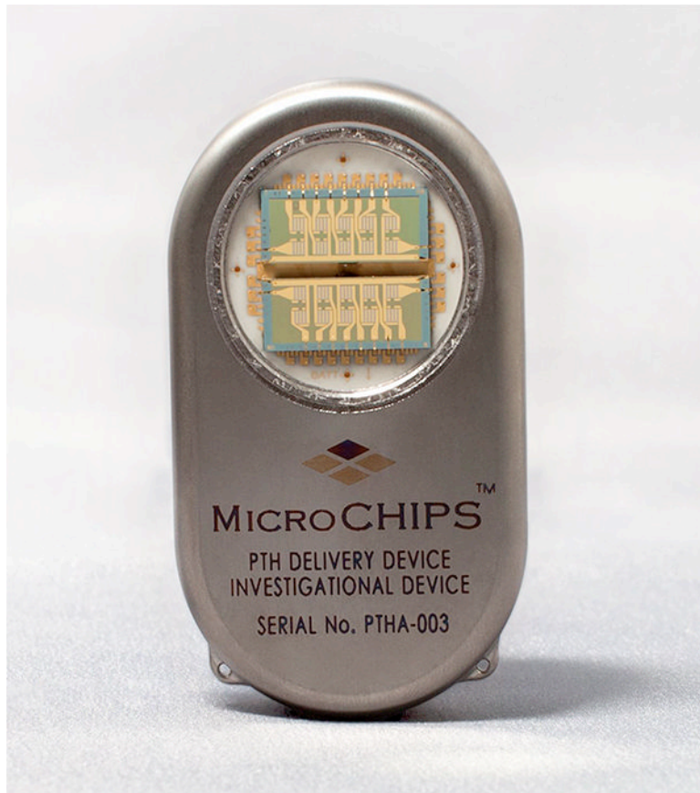
Figure 17. MicroCHIPS Drug delivery device. Courtesy of MicroCHIPS, Inc.
