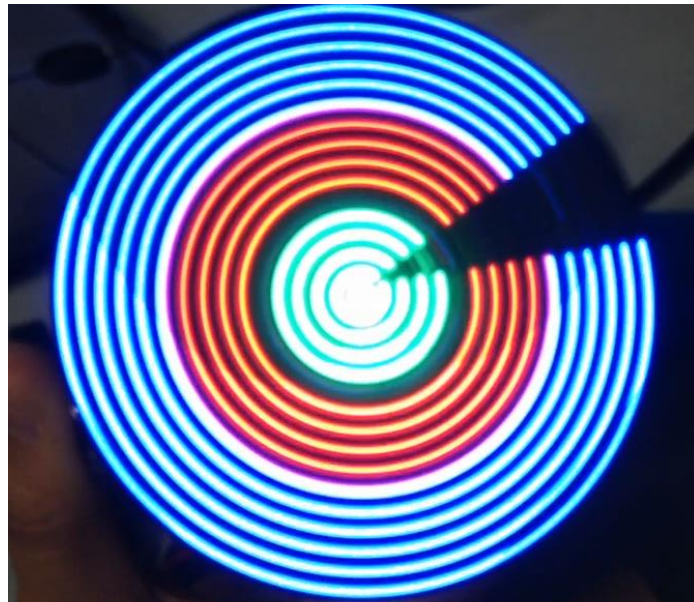
Figure 11. Image of PCB spinning at 40.3Hz displaying RGB Pac-Man
