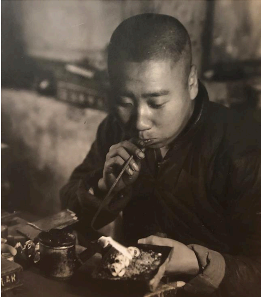
Fig. 3.30. Beijing silversmith using a blowpipe. From Hedda Morrison, “Handicrafts” albums, photographs taken in Beijing ca. 1933-1946. Yenching Library, Harvard University
