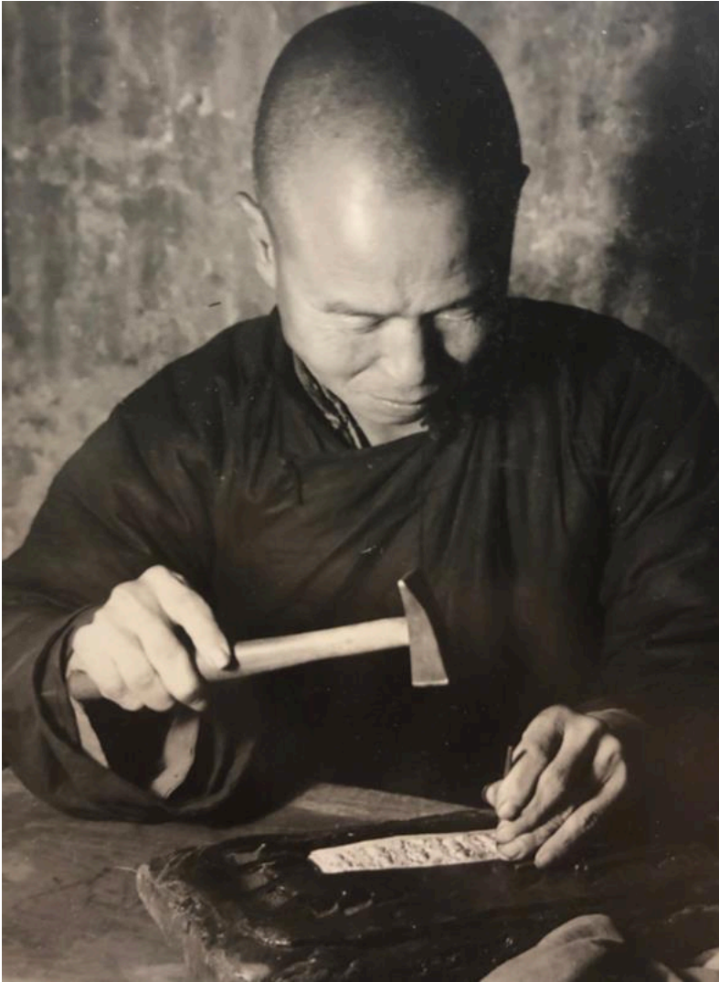
Fig. 3.29. Beijing silversmith embossing a piece of silver with a hammer and punch. From Hedda Morrison, "Handicrafts" albums, photographs taken in Beijing ca. 1933-1946. Yenching Library, Harvard University
