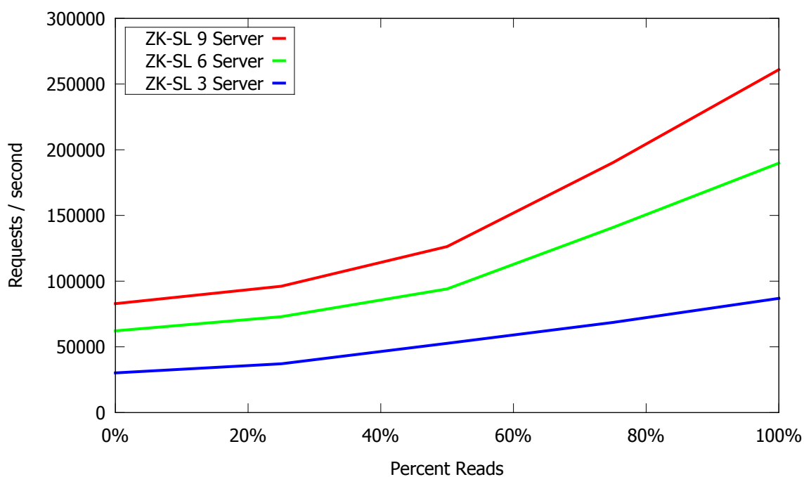
Figure 6.3. ZooKeeper-SL Requests per Second. Requests per second as a function of read percentage on ZooKeeper-SL. In our shared log implementation, the write throughput (on the left) scales as the number of translation servers increases. The read throughput (on the right) scales similarly to ZooKeeper.
