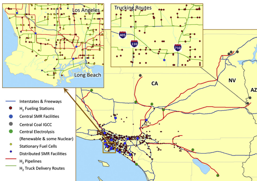
Fig. 1 – Spatial allocation of Scenario H implemented for the South Coast Air Basin of California (SoCAB). Geographic information systems (GIS) data are utilized to determine realistic sites for various components of hydrogen infrastructure at a high level of spatial and temporal resolution. Screening criteria applied in the analysis include proximity to existing fueling stations, hydrogen generation facilities, electrical power plants, roads and pipelines, density of hydrogen fueling stations, land use characteristics, and wind and solar resources. Routes for distribution of hydrogen by truck and pipeline were allocated using best route algorithms.
