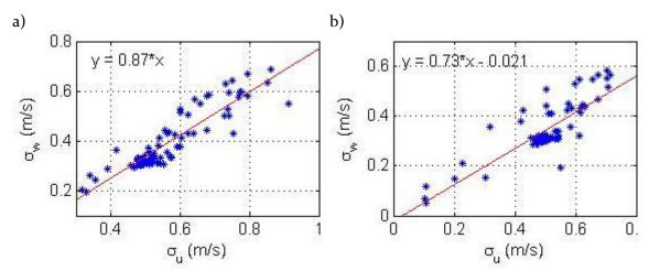
Figure 3-6- Scatterplots comparing  $\sigma_u$  values with  $\sigma_w$  values at different points within the wind tunnel for a) solid barrier case, and b) vegetation case.
