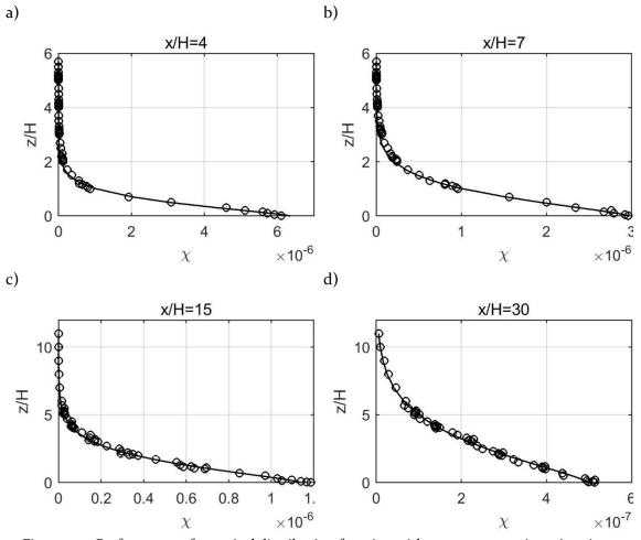
Figure 4-7- Performance of a vertical distribution function with exponent s=1.3 in estimating vertical concentration profiles of the FLAT case at different downwind distances.
