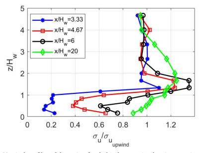
Figure 3-9- Vertical profiles of the ratio of  $\sigma_u$  behind vegetation barrier to  $\sigma_u$  in undisturbed boundary layer. The vegetation extends from  $x = 2H_w$  to  $x = 3H_w$ .
