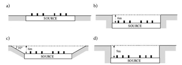
Figure 4-2- Elevation view showing cross sections through the different roadway designs studied; a) flat terrain roadway (FLAT), b) 6 m deep depressed roadway with vertical sidewalls (D690), c) 6 m deep depressed roadway with 30° sloping sidewalls (D630), and d) 9 m deep depressed roadway with vertical sidewalls (D990). The small black rectangles indicate the location of the tracer emission lines. The width of the road in all cases is 36 m. Adapted from Heist et al. (2009).
