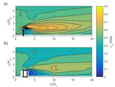
Figure 3-5- Contours of longitudinal velocity fluctuations for a) solid barrier case and b) vegetation barrier case. Barriers are represented by black rectangles.
