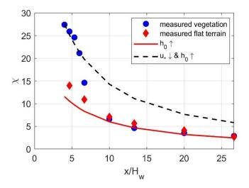
Figure 3-11- Comparison of the measured surface concentrations with estimated surface concentrations versus downwind distance. Vegetation ends at  $3H_w$ .
