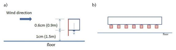
Figure 3-2- Schematic of the line sources in the wind tunnel study; a) looking crosswind, and b) looking upwind.
