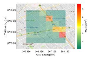
Figure 5-13 the plot of estimated daily-averaged primary PM2.5 concentrations due to line sources within the 3-km grid.
