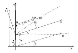
Figure 2-1- Co-ordinate systems used to calculate contribution of point source at  $Y_s$  to concentration at  $(X_r, Y_r)$ . The system x-y has the x-axis along the mean wind direction, which is at an angle  $\theta$  to the fixed X-axis. Adapted from (Venkatram and Horst, 2006).
