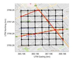
Figure 5-12- The line sources detected within the grid (indicated by red lines). The red circles indicate the traffic sensors available in AADT files
