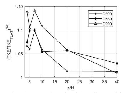
Figure 4-5- Gradient of square root of TKE values of a) D690, b) D630, and c)D990 cases, normalized by the corresponding values observed at flat terrain case.
