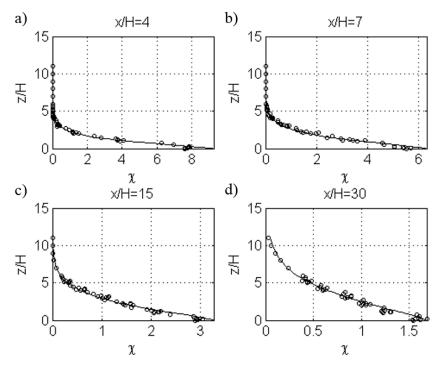
Figure 4-10- Comparison of the vertical concentration profiles at multiple downwind locations predicted by the modified van Ulden model (with s=1.3 and p=1/4) with those of the observations (D690 case).
