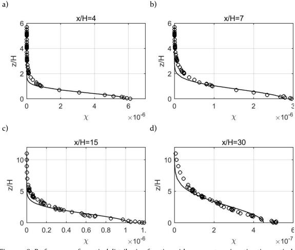
Figure 4-8- Performance of a vertical distribution function with exponent s=2 in estimating vertical concentration profiles of the FLAT case at different downwind distances.
