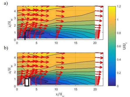
Figure 3-3- Magnitudes of observed velocity and velocity fields for a) solid barrier case and b) vegetation barrier case. Barriers are represented by black rectangles.
