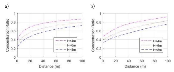
Figure 2-15- Comparison of estimated normalized concentrations, to no-barrier case, behind barriers with different heights for a) simple barrier model and b) the modified mixed-wake model.
