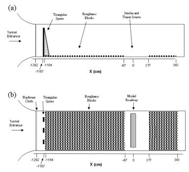
Figure 4-1- Schematic of near roadway wind tunnel setup: a) elevation and b) plan view.
