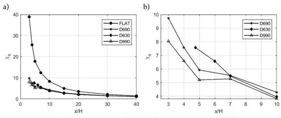
Figure 4-6- Surface concentration as a function of downwind distance for different road configurations. Left plot includes flat terrain concentrations.
