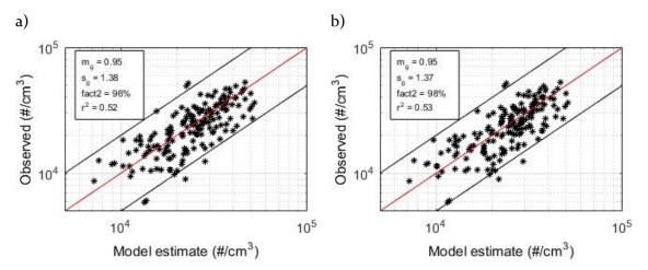
Figure 2-12- Comparison of observations and a) simple barrier model estimates and b) the modified mixed-wake model estimates.
