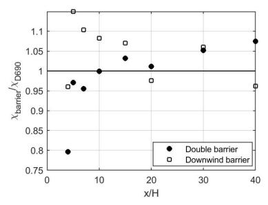
Figure 4-14- Ratio of surface concentrations downwind of barrier cases to those of D690 case. (Solid circle corresponds to 6 m double solid barriers and open square corresponds to 6 m downwind barrier).
