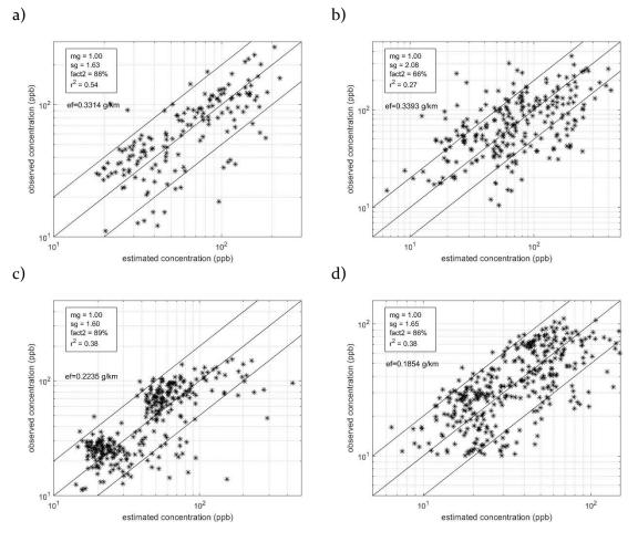
Figure 5-8- Comparison of NOx observed concentrations and simple line source model estimates during a) winter unstable, b) winter stable, c) summer unstable, and d) summer stable. Emission factors are shown on each plot.
