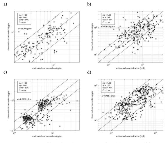
Figure 5-10- Comparison of NOx observed concentrations and simple line source model estimates during a) winter unstable, b) winter stable, c) summer unstable, and d) summer stable. Emission factors are shown on each plot.
