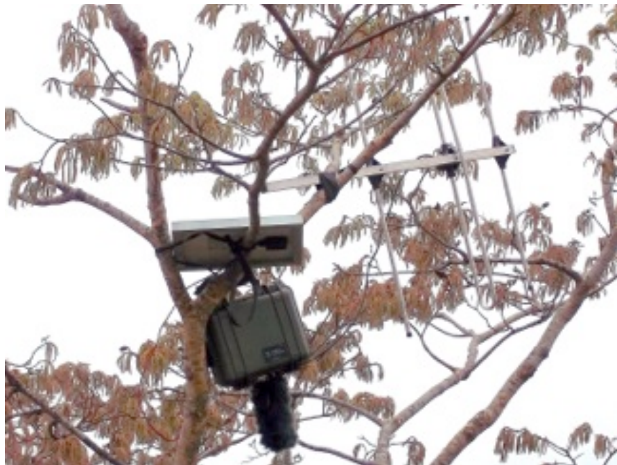
Figure 9 - A solar powered acoustic transmission unit (SPATU) deployed in the Issa Valley
