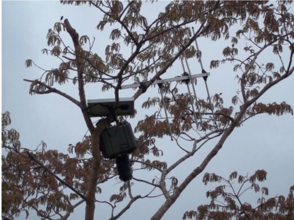
Figure 19 - A solar powered acoustic transmission unit (SPATU), deployed in the Issa Valley.
