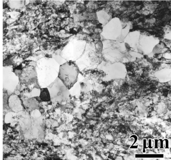
Figure 1.2 | TEM image of Ti with heterogeneous lamella structure, showing a lamella of recrystallized grains in between two lamellae of ultra-fine grains.
