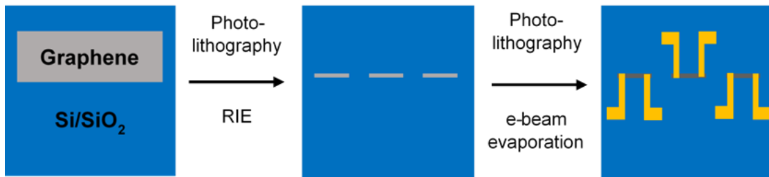
Figure 4.3 Process flow diagram for fabrication of graphene-FETs using photolithography.
