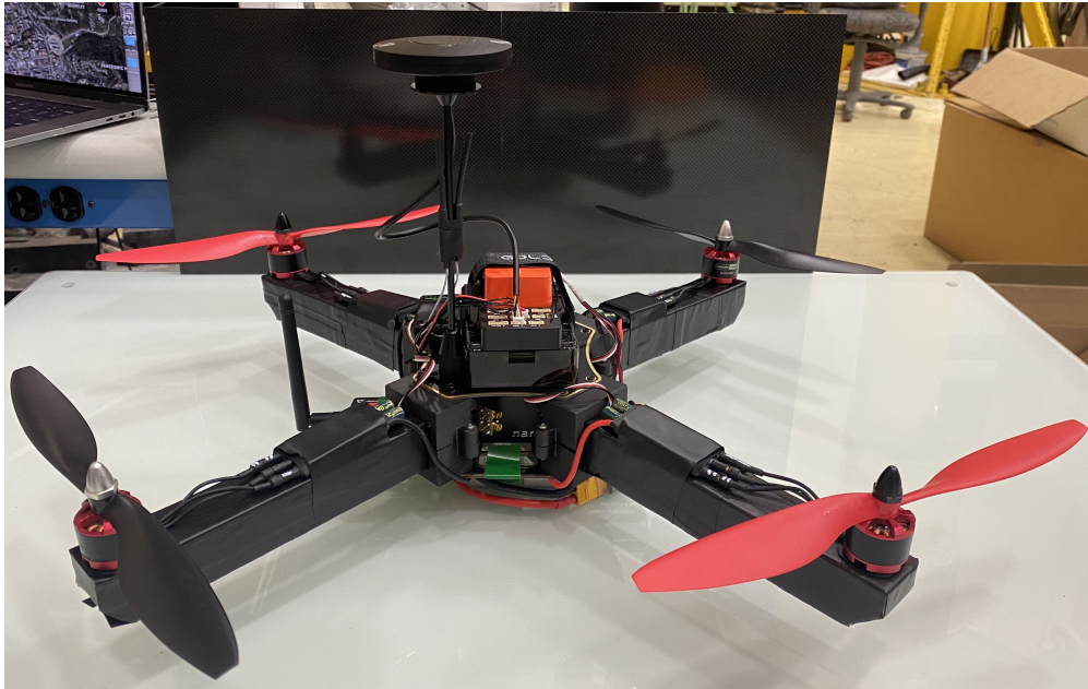
Figure 7.1: Initial sUAS prototype consisting of 7.5-inch long structural PSD plastic scintillator frame component arms
