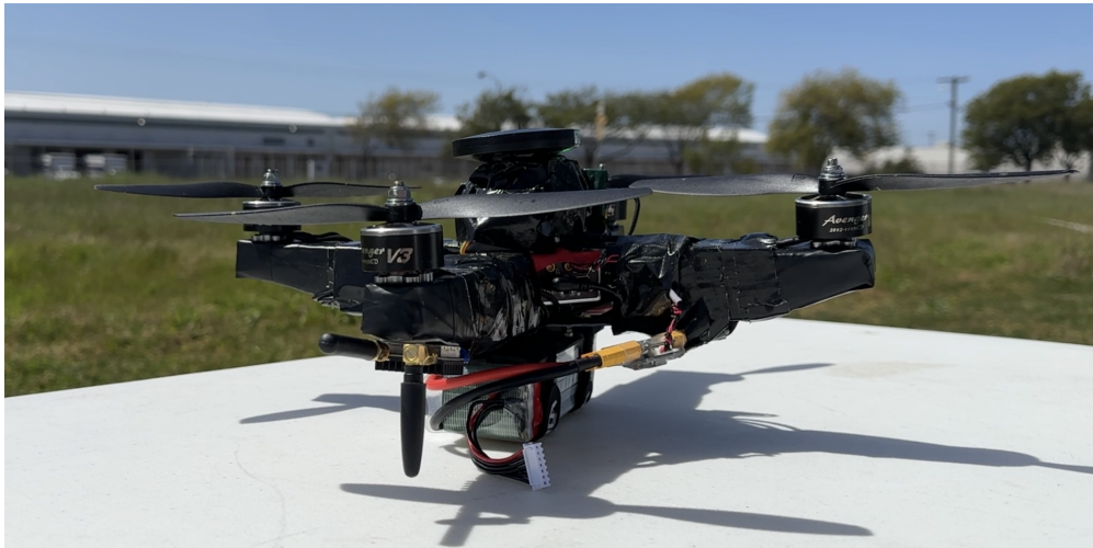
Figure 5.9: Photo of assembled sUAS with RFD900x telemetry module in the foreground
