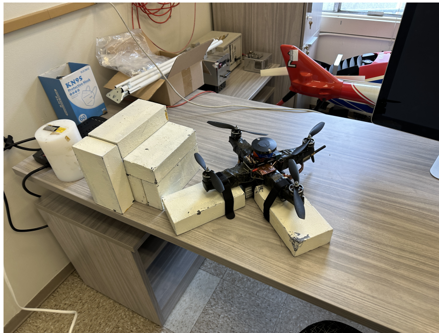
Figure 7.15: Laboratory PSD characterization setup for assembled sUAS
