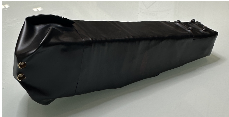
Figure 5.6: Photo of optically-sealed PSD plastic structural sUAS component assembly
