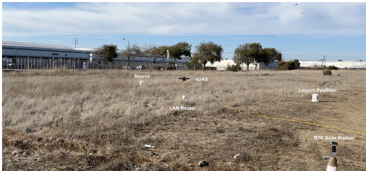
Figure 7.4: Photo of initial prototype field measurement demonstrating the sUAS in flight, with locations depicted of the mixed \gamma -n source, launch position, LAN router, and RTK base station, from the visual perspective of the GCS.
