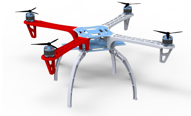
Figure 4.13: CAD model of DJI F450 sUAS platform [34]
