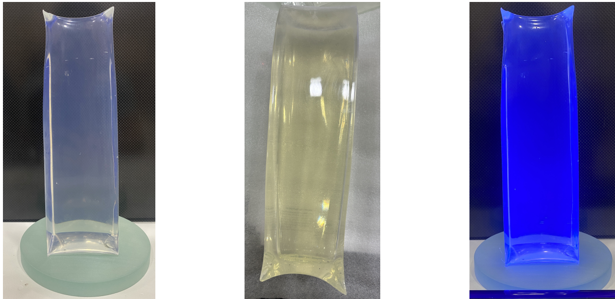
Figure 5.1: Left: Photo of bulk scintillator material block, composition 1. Center: Photo of bulk scintillator material block, composition 2. Right: Photo of bulk scintillator material block, composition 1, illuminated by UV lamp.
