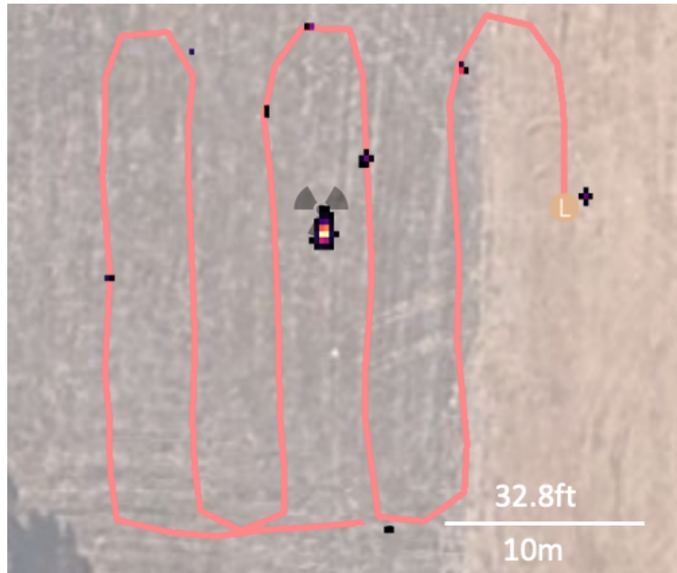
Figure 7.12: Overlaid comparison of the reconstructed source location pixels to the true source location indicated by the trefoil, reference to the measurement path line in red
