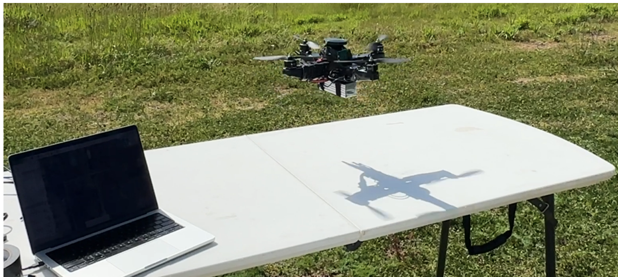
Figure 7.14: Photograph of second-generation sUAS prototype, composed of 4.5-inch structural PSD plastic frame arm components, in guided flight
