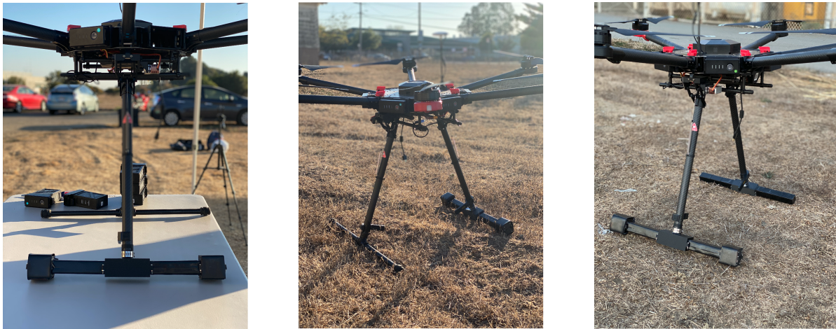
Figure 3.19: Photos of LBNL operated DJI Matrice 600 sUAS platform depicting the replacement of a landing foot with a structural PSD plastic detector assembly (left, center), as well as the replacement of the second carbon-fiber foot with a PMMA 16” long 1” x 1” square rod (right)
