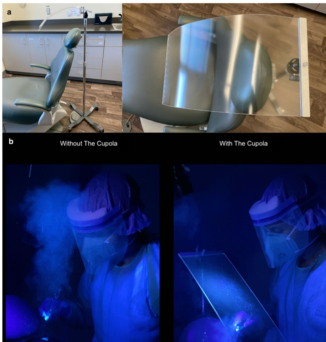
Fig. 1 a The Cupola—protective shield. b Simulated dental procedure using a high-speed handpiece without and with The Cupola
