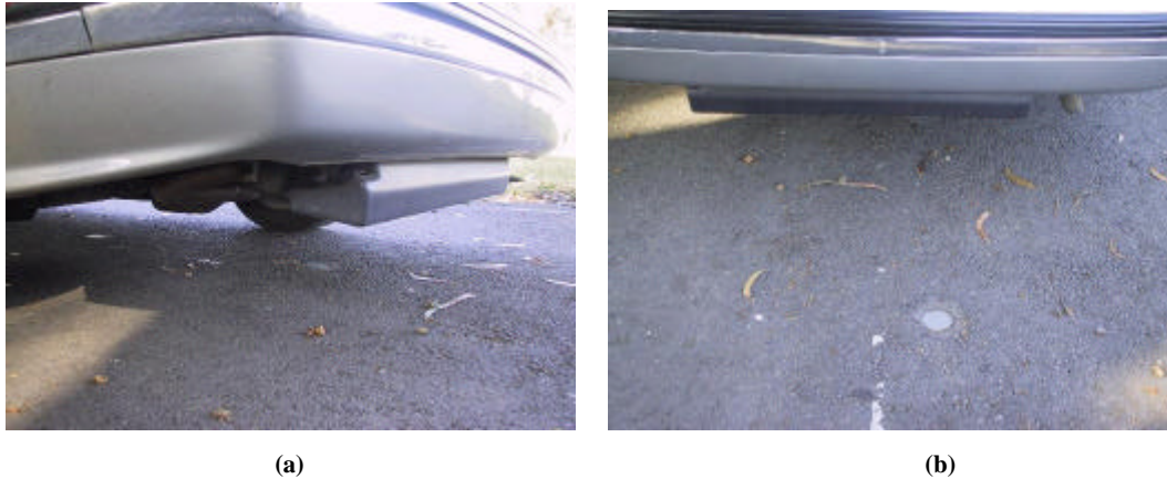
Fig. 4.5: Magnetometers mounted on the front (a) and rear (b) bumper
