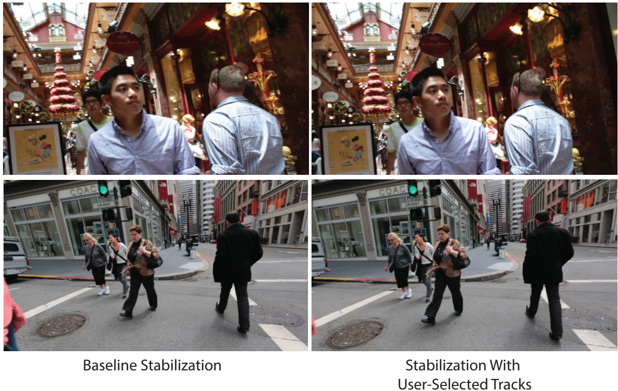
Figure 5.7: Comparison of initial baseline with result using user-selected tracks. The face and torso of the subject have less horizontal stretch in the top example. The walls of the buildings on the left are less skewed in the bottom example.
