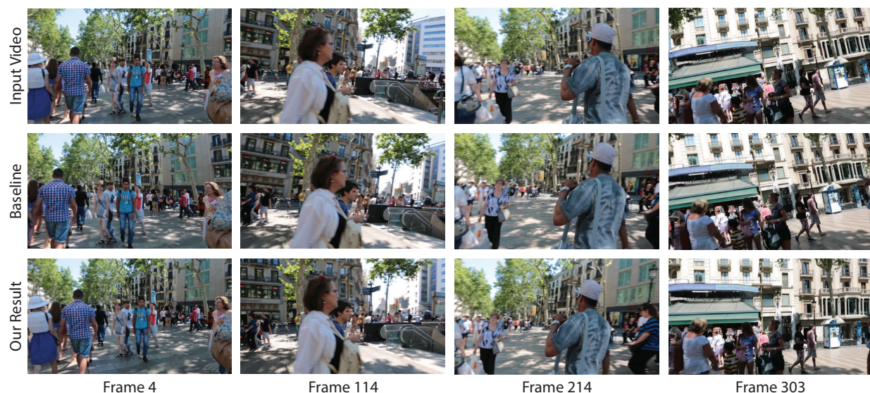
Figure 5.10: Notice that in our result, frame 4, 114 and 214 have facades that are more vertical compared to the baseline stabilization. In particular, the baseline stabilization did not correct for the slow rotation for the camera in frame 303 while our method corrects for it as the user specified that the rotation should be removed.
