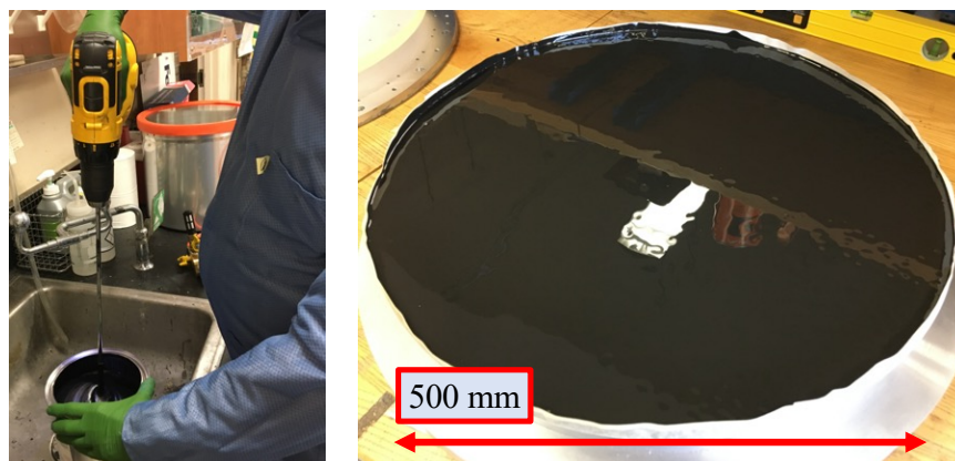
Figure 10.8: Photographs of the epoxy AR application and cure. The left photo is of the epoxy resin being mixed in the can to evenly distribute the fillers. The right photo is of the epoxy mixture on the sapphire’s surface right after application. It is coated all the way to the edge, and a barrier of masking tape keeps the epoxy from leaking over the edge. A leveling table keeps the layer flat as it cures.
