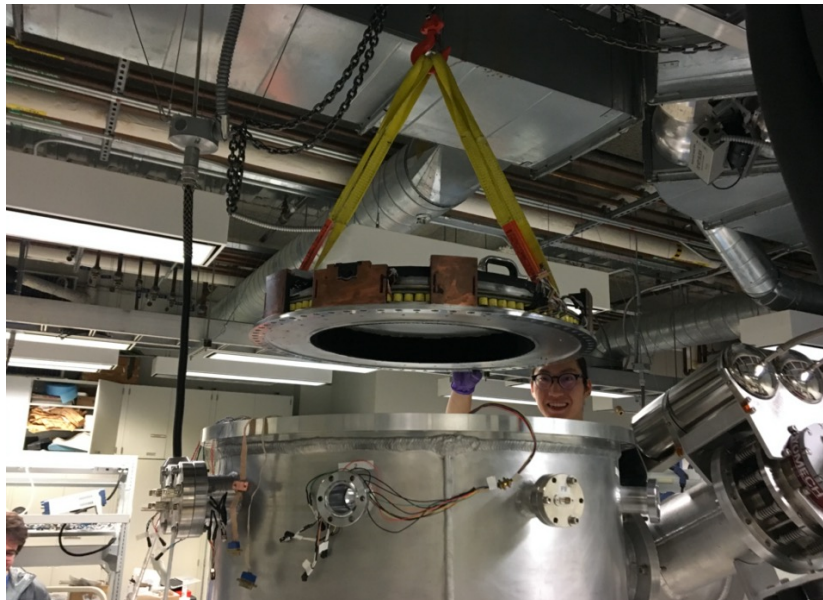
Figure 8.12: A photo of the CHWP being installed into the PB-2b optics tube. The cryostat is constructed vertically on a cart from the focal plane towards the sky. The CHWP is one of the last elements to be installed and is hoisted using a series of handles that attach to the rotor stage. Once above the receiver, the CHWP is slowly lowered into the optics tube and is bolted to the 50 K stage.
