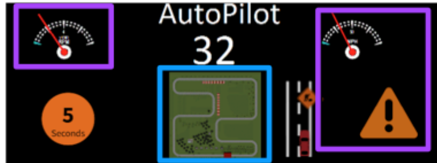
Figure 4.8: User Interface Used in Study. The base interface (UI1) includes the control mode, time to transfer, scene visualization and speed. UI2 includes the basic features as well as navigation as seen in the blue box. UI3 builds off of UI2 and includes an RPM gauge, speedometer, and warning icon, as seen in the purple boxes.
