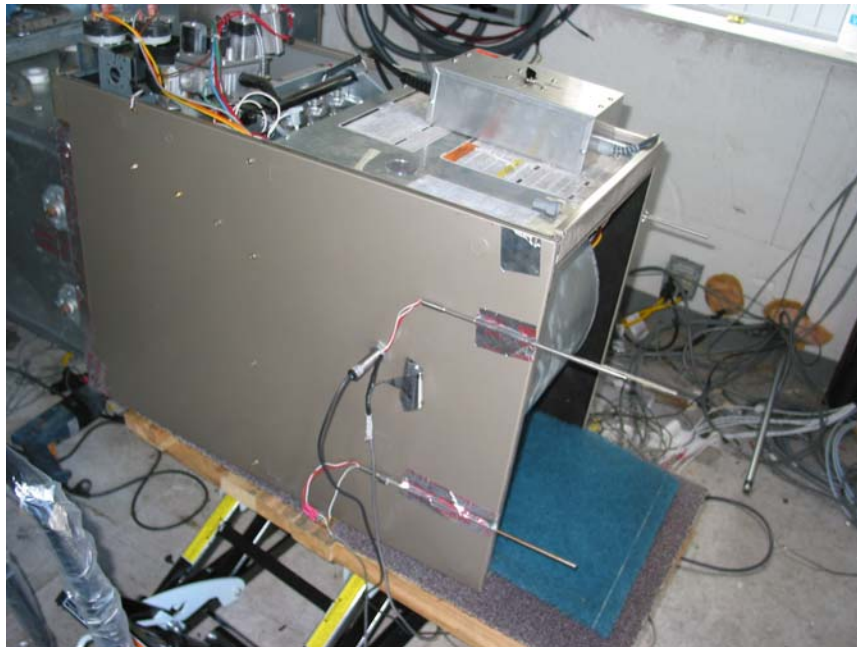
Figure 13. Furnace mounted in electric utility test apparatus
