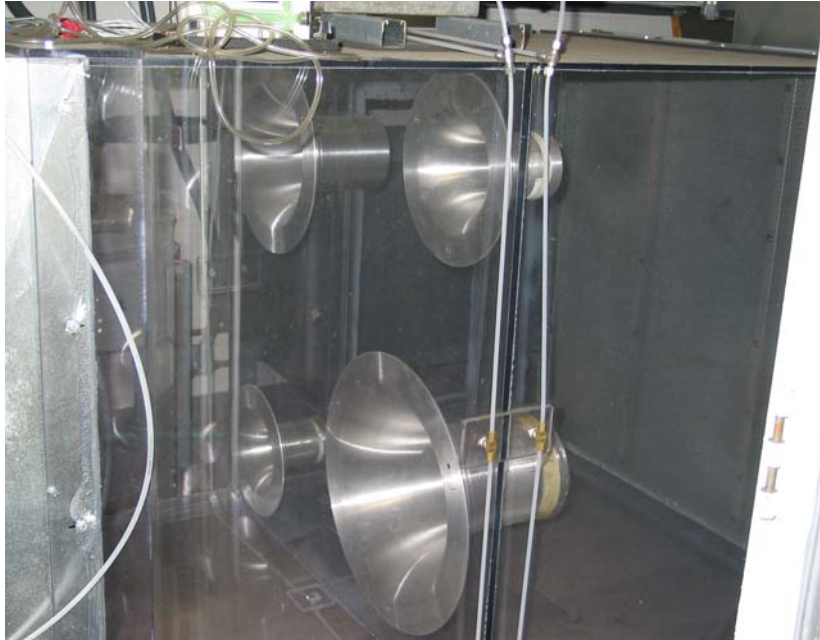
Figure 14. Flow nozzles in electric utility test apparatus
