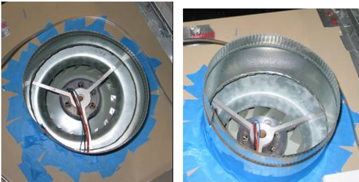
Figure 10. Fabricated Motor Side entry for Furnace #1
