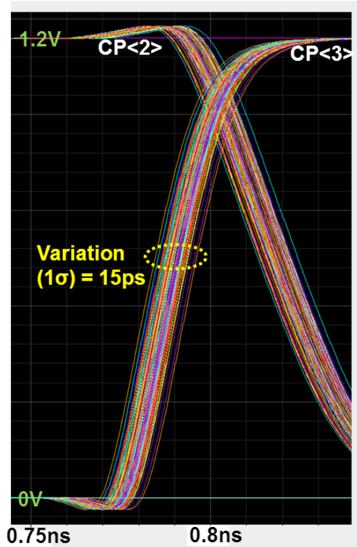
Figure 4.19: Monte-Carlo simulation of post-layout extracted CP \langle 2 \rangle , CP \langle 3 \rangle at 5GS/s.
