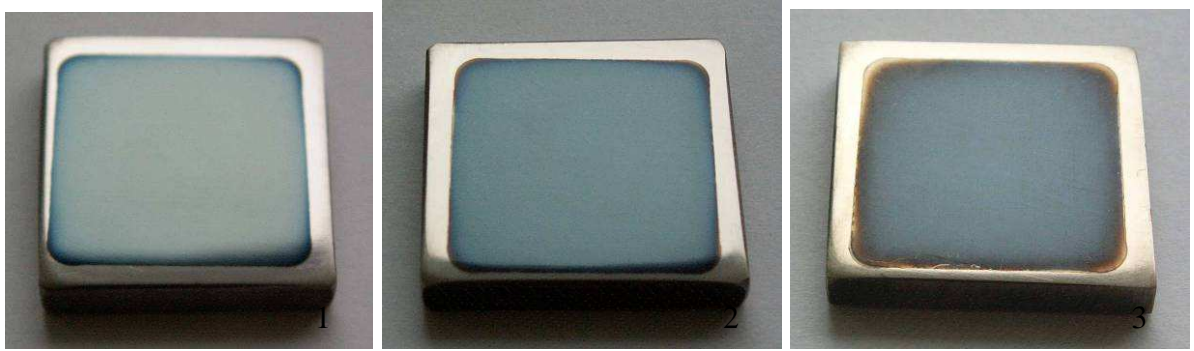
Fig. 46. DLC film on the HSS specimen. Amplitude of negative bias voltage in DLC film deposition: -10 kV (1), -15 kV (2), -20 kV (3).
