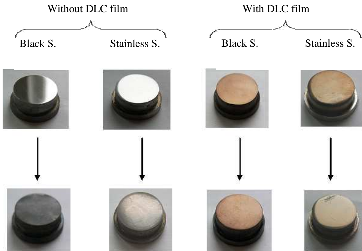
Fig. 52. Specimens with and without DLC films attacked by concentrated sulfuric acids. The upper row – before the attack, the low row - after 30 min of effect.
