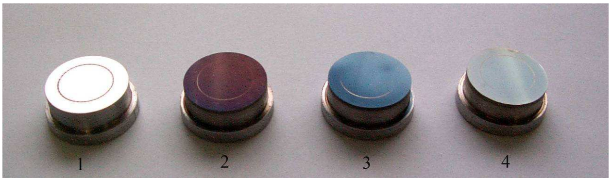
Fig. 30. Specimens for tribological measurements: without film (1), U_{\text{bias}} = -10 kV (2), U_{\text{bias}} = -15 kV (3), U_{\text{bias}} = -20 kV (4).
