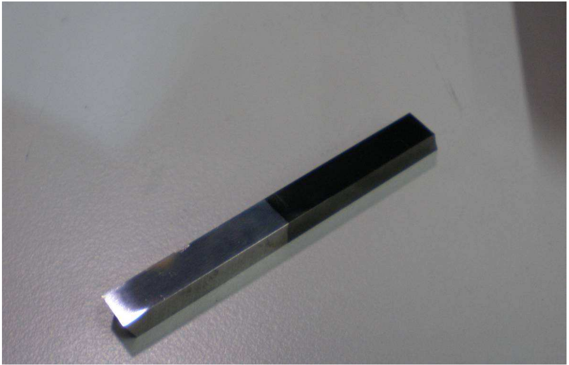
Fig. 69. High-speed steel specimen with a DLC coating.
