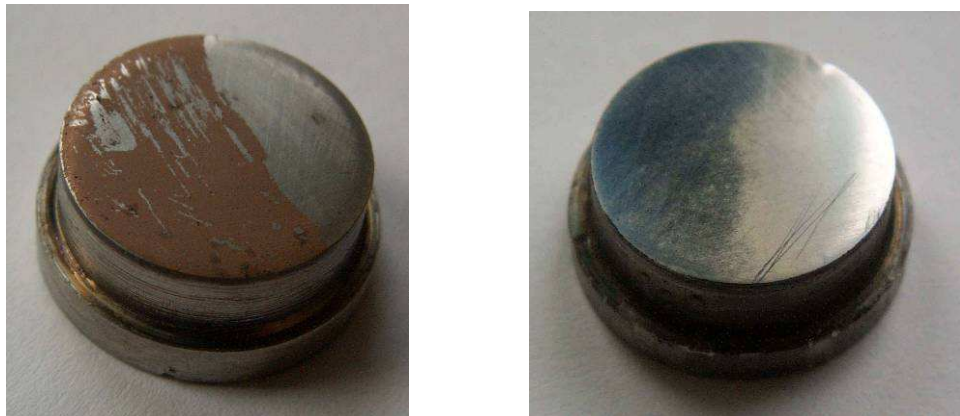
Fig. 27. Films deposited on the SS surface in the low-voltage mode.
