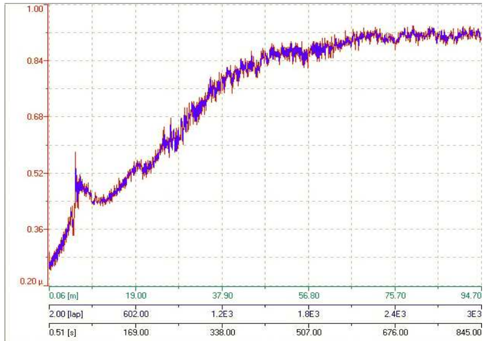
Fig. 31. Friction coefficient of the initial SS specimen without DLC film.
