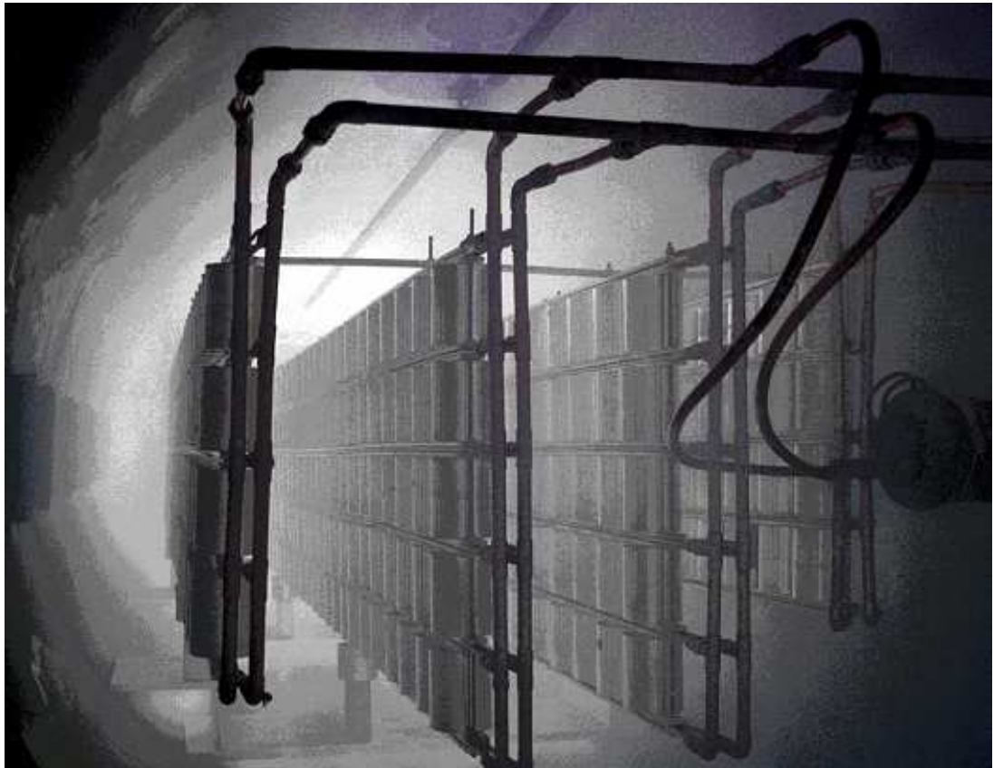
Fig.9. Plasma cleaning, ion implantation, and DLC deposition of 1000 automotive pistons in the former OFES facility (Los Alamos National Lab.)
