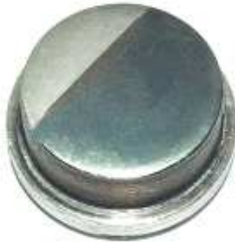
Fig. 41. DLC film on the nitrated SS surface. (During the deposition, the upper corner of the specimen was shielded).
