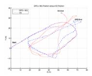
Motion estimate using Visual Odometry alone. 14.7 meter error over 405.5 meters.
