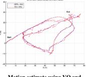
Motion estimate using VO and IMU data. 1.6 meter error over 405.5 meters.
