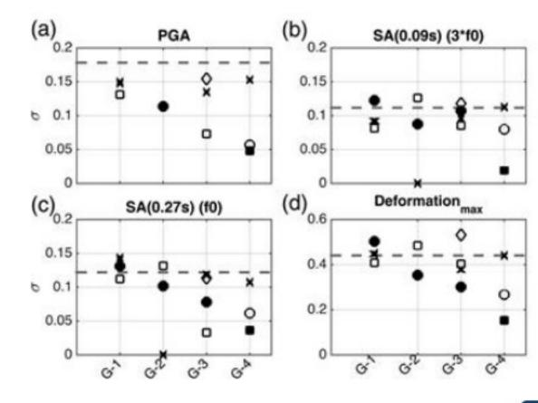
Standard deviation values ( $\sigma_{log}$ , in  $log_{10}$  units) of four parameters for the NL comotion scaled to the highest PGA: (a) RS at 0.27 s, (b) RS at 0.09 s, (c) all three at shear deformation at the bottom of P1. The standard deviations are given for eatheir low-strain attenuation implementation (G-1), their numerical scheme (G-2) their values of shear strength at the bottom of P1 and use of damping control or illustrates the standard deviation for all code/team couples.
