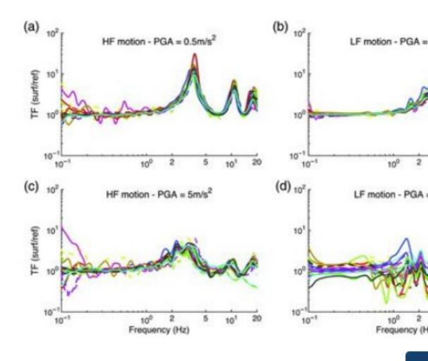
Comparison of the surface to reference Fourier spectra ratio, for the nonlinear (N motion (a) scaled to 0.5 m/s<sup>2</sup> and (c) scaled at 5 m/s<sup>2</sup>, and using the LF input moti (d) scaled at 5 m/s<sup>2</sup>.
