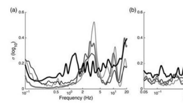
Standard deviation (in log unit) of the (a) transfer function and (b) response specused.
