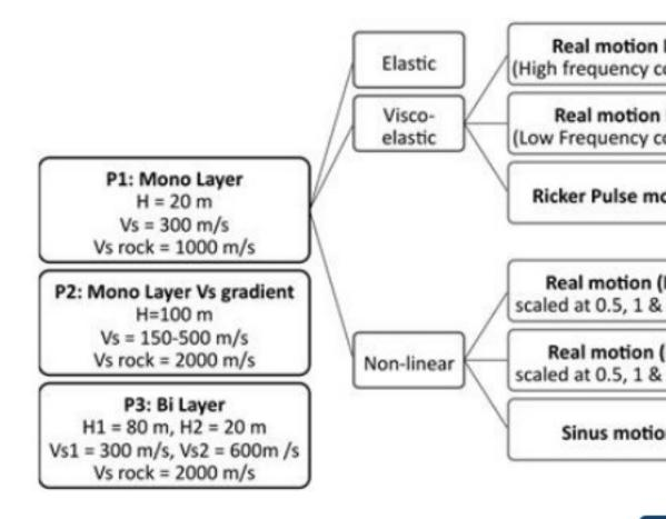
The three simple idealized profile cases studied here (P1-P3), for the elastic and elastic soil-bedrock base, using a Ricker pulse and three accelerations of differer frequency contents.
