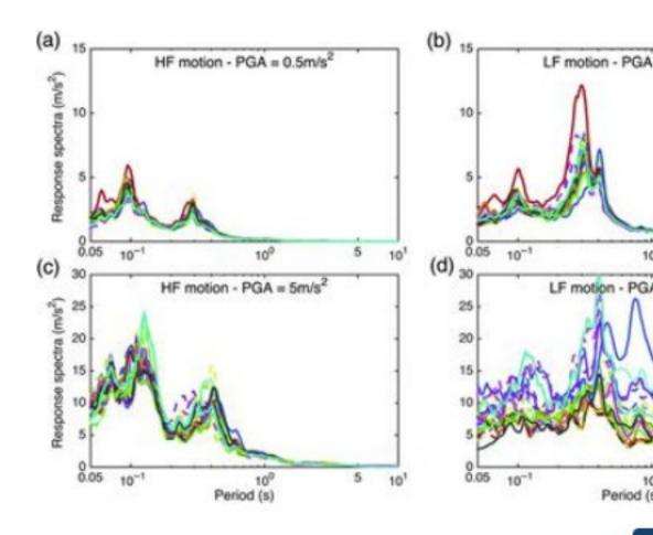
Comparison of the acceleration pseudoresponse spectra at the ground surface, input motion (a) scaled to 0.5 m/s $^2$  and (c) scaled at 5 m/s $^2$ , and using the LF input motion at 5 m/s $^2$ .
