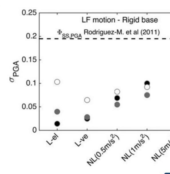
Standard deviation (in log unit) of PGA for profiles 1, 2, and 3, for the five differe linear-viscoelastic, NL with input motion scaled to the lowest).
