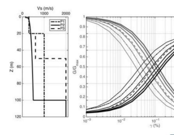
$V_S$  profiles,  $G/G_{max}$ , and damping curves for the three idealized profiles.
