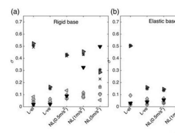
Standard deviation (in log unit) of the different intensity parameters for the P1 computational cases: linear–elastic, linear–viscoelastic, NL with input motion (1  $\text{m/s}^2$ ), and highest (5  $\text{m/s}^2$ ) PGA, for the LF content motion. (a) The results elastic substratum.
