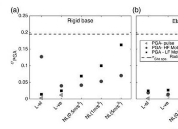
Standard deviation (in  $log_{10}$  unit) of PGA at the surface of the P1 profile, for the linear-elastic; linear-viscoelastic; NL with input motion scaled to the lowest (0.5 m/s<sup>2</sup>) PGA, for the pulse-like, the HF and LF content motions. (a) The results f (b) the elastic substratum.
