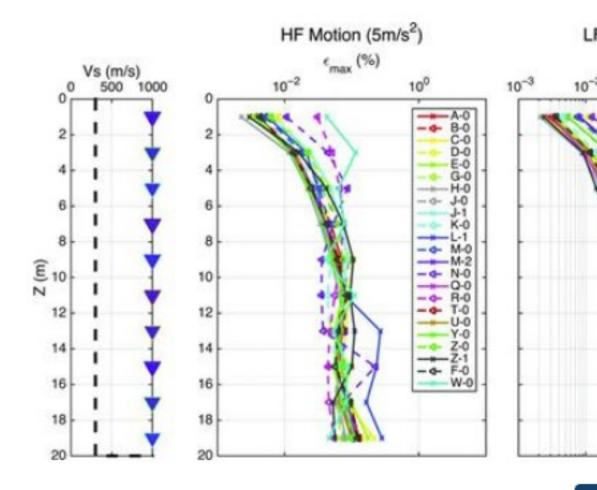
Peak shear-strain profiles reached at each depth by each team for the HF and LF PGA level (5  $\,$  m/s $^2$ ), for profile 1 and for rigid substratum conditions.
