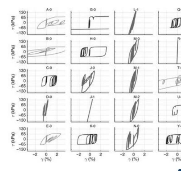
Stress-strain curves at the bottom of the P1 profile for the rigid substratum cases the highest PGA [5 m/s<sup>2</sup>]). The thicker curves are for code/team couples that e 65 kPa, whereas the thin curves represent the code/team couples that use 65 k using damping control and the darker curves the others.
