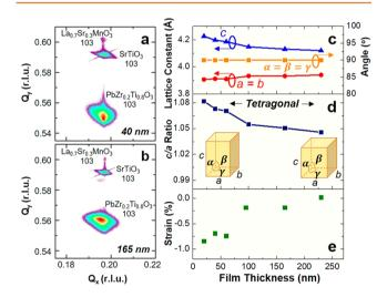
Figure 2. X-ray reciprocal space mapping studies of the 103diffraction conditions of films and substrates for (001)-oriented  $PbZr_{0.2}Ti_{0.8}O_3$  heterostructures of thickness (a) 40 nm and (b) 165 nm. Thickness dependence of (c) lattice constants and interaxial angles, (d) c/a ratio, and (e) self-strain in (001)-oriented heterostructures.
