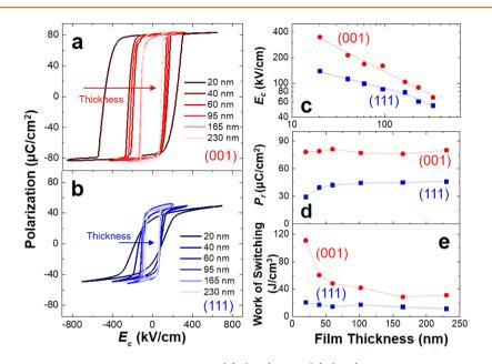
Figure 1. Ferroelectric hysteresis loops measured at 1 kHz for (a) (001)- and (b) (111)-oriented heterostructures as a function of film thickness. (c) Coercive field  $(E_c)$ , (d) remanent polarization  $(P_r)$ , and (e) work of switching plotted as a function of film thickness for (001)- and (111)-oriented heterostructures.
