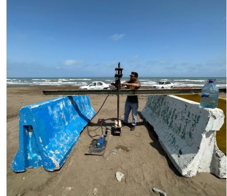
735 Fig. 16 Site testing: (a) Installation procedure; (b) Compression testing setup; (c) Pullout testing 736 setup
