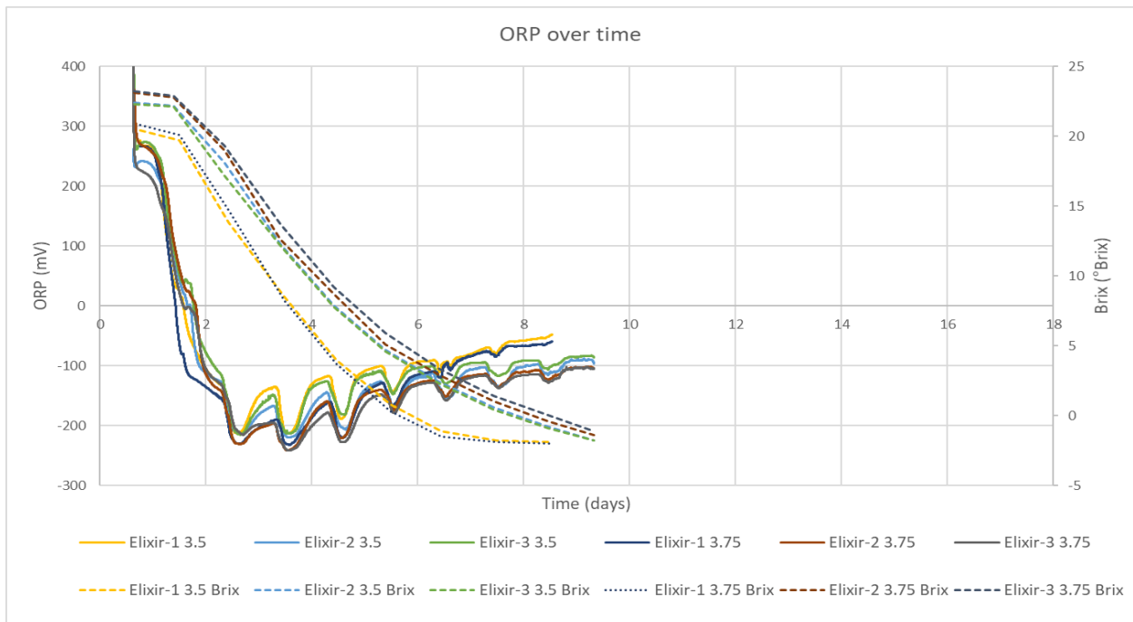
Figure 3.4.7: ORP curves for Elixir yeast at pH 3.5 and 3.75. Initial conditions start at about 21°B at a temperature of 23 °C. Bioreactor trial number for each replicate found in Table 3.4.2.
