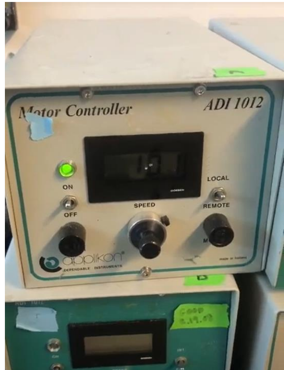
Figure 2.1.5: Image of bioreactor motor control box.
