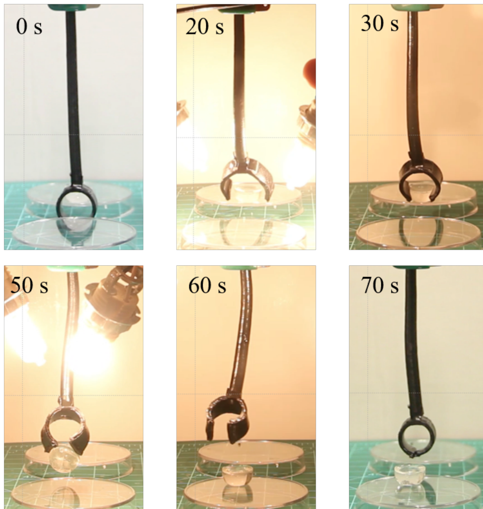
Figure 3.5: Soft gripper prepared from LCE-CNT rod and LCE-CNT arch structure. The soft gripper can fully light-driven gripping and manipulation which enables moving a PDMS piece from the rear to the front plate.
