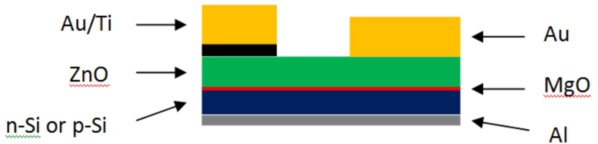
Fig. 2.1: Mixed view of the structures of all fabricated samples
