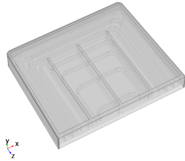
Figure 5.13: WCLL BB CAD model
