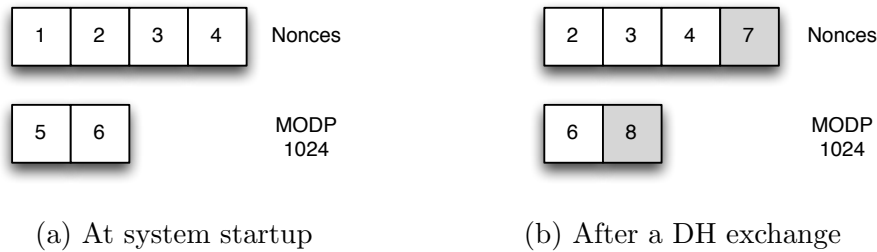
Figure 2.1: Nonce queue behavior during an IKE handshake.
