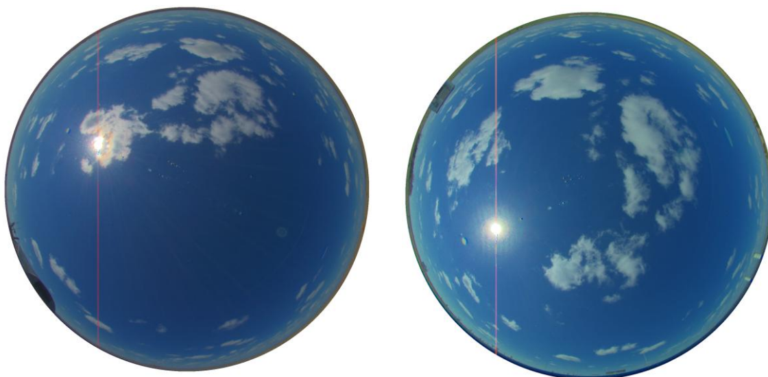
Figure 5.2. Image pairs for which a dense estimation of cloud position was performed. Images on the left are from USI 1.7 (note Farmer Bobbit's roundtop barn), and images on the right are from USI 1.8. All images are color corrected HDR with a logarithmic intensity rescaling (similar to gamma correction). ( continued )
