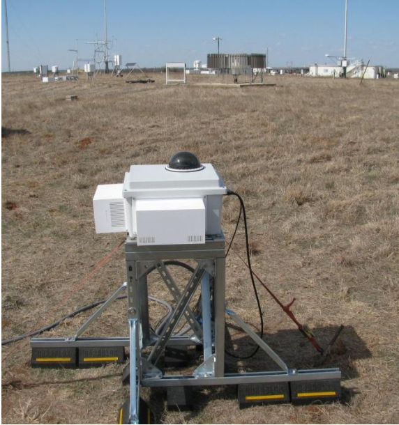
Figure 3.1. USI 1.8 in the instrument field at the Department of Energy, Atmospheric Radiation Measurement Program, Southern Great Plains Climate Research Facility.
