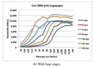
Figure 3. Sandia MPI Micro-benchmark *msgrate* results on Cori. Using 2 MiB pages improves performance substantially for message sizes > 8 KiB.
