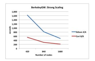
Figure 11. BerkeleyGW strong scaling charateristcs using the best MPI/OpenMP combinations
