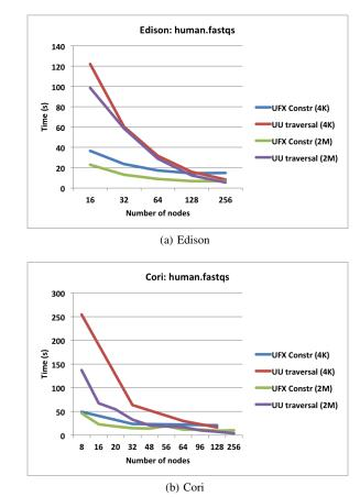
Figure 14. Strong scaling with 24 UPC threads (Edison) and 64 UPC threads (Cori) per node using the human.fastqs dataset.
