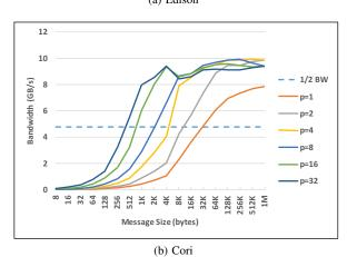
Figure 4. UPC uni-directional "put" bandwidth. "Get" bandwidths (not shown) are similar, but are 10% lower for all message sizes and pair counts.
