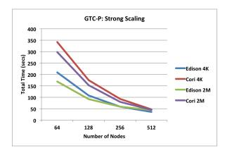
Figure 13. GTC-P strong scaling charateristcs using the best MPI/OpenMP combinations
