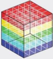
**Snapshot or non-scanning imaging** simultaneously captures both spectral and spatial information in a single image ( $x, y, \lambda$ ) over a single integration time—using, for example, a large-format detector array capturing different wavelengths. No scanning is involved, so motion artifacts are eliminated and data processing simplified. That makes the technique ideal for low-resolution video rates, low-light imaging or high-speed applications.
