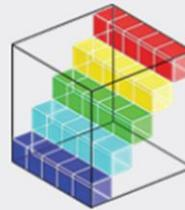
**Spatio-spectral scanning** acquires a series of thin diagonal ( $x, y$ ) slices of the data cube, each at every wavelength in the series. Typically, the system or camera must be scanned transverse to the slit. The dispersion-based system yields high spectral and spatial resolution, which is useful in astronomical imaging.
