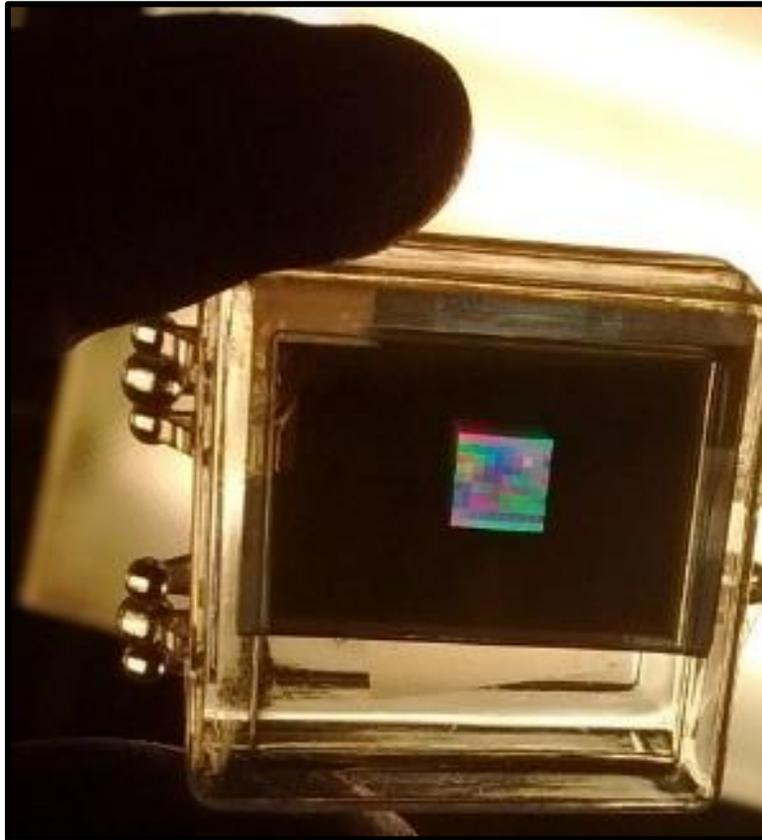
*Figure 1.2: 10 by 10 array of etalons of size 500 by 500 microns for reconstructive spectrometry in the visible wavelength region.*
