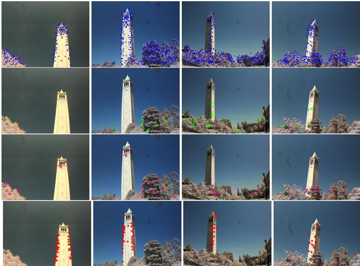
Figure 3.1: Comparison of informative feature selection on low-quality multiple-view images. Top: A subset of 16 training images of a building (Campanile at UC Berkeley) in the BMW database [67] with SURF features superimposed in blue. Middle-top: Informative features detected by SfM (green). For each image pair, SURF features are deemed informative if the consensus of the corresponding epipolar constraint exceeds 25% of the total feature pairs. Middle-bottom: Informative features selected by thresholded PCA (pink), with desired cardinality equal to that of Sparse PCA. Bottom: Informative features selected by Sparse PCA (red) based on the first two leading PVs. The selected features primarily lie on the Campanile, while other features on the trees, lamps, and other objects are successfully suppressed. For this particular dataset, the SfM method performs poorly due to unreliable epipolar transformations found between these wide-baseline images.
