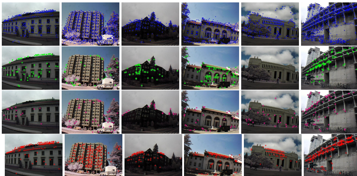
Figure 3.4: Top: Images of 6 objects in the BMW database with superimposed SURF features; Middle-top: Informative features detected by the SfM approach; Middle-bottom: Informative features detected by thresholded PCA; Bottom: Informative features detected by Sparse PCA (given by first two leading sparse PVs).
