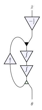
Note that this already includes a kind of feedback loop, since the pendulum's angle affects the force on the pendulum.
