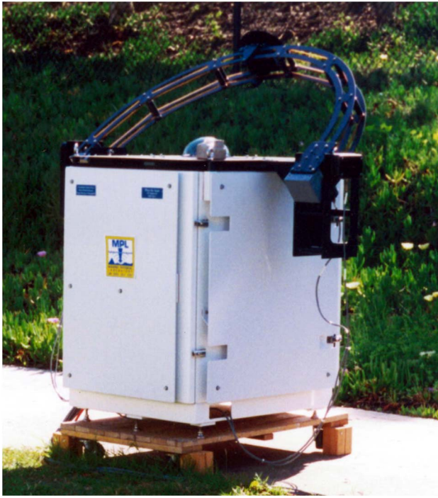
Fig. 3. (Color online) D/N WSI developed at MPL starting in the early 1990s.
