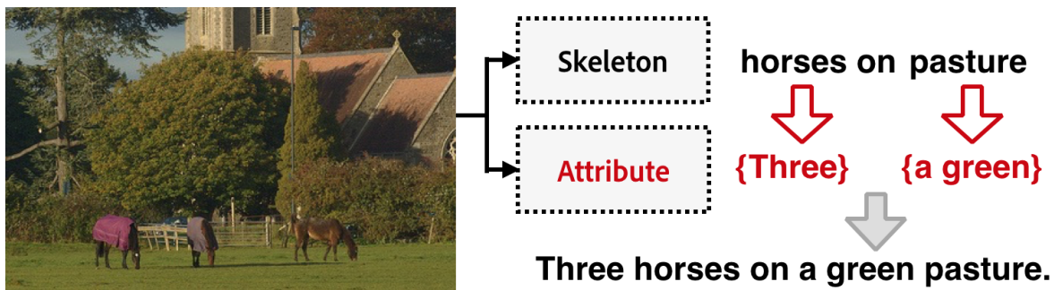
Figure 4.1: Illustration of the inference stage of our coarse-to-fine captioning algorithm with skeleton-attribute decomposition. First, the skeleton sentence is generated, describing the objects and relationships; Then, the objects are revisited and the attributes for each object are generated.
