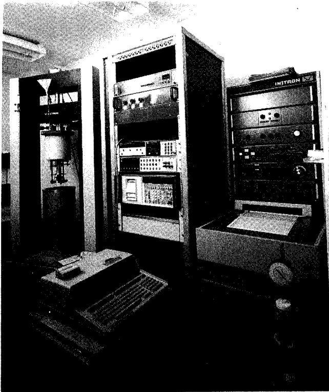
Mechanical facility for compression and thermal tests (400 to 4 K).
