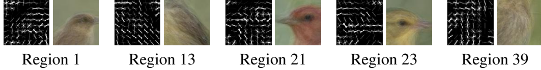
Figure 4.4. Discovering Discriminative Regions. We discover a set of discriminative regions (Section 4.4) and select a subset to use in our experiments, each visualized above as a HOG template alongside the averaged image of the highest confidence positive detections for that corresponding detector.
