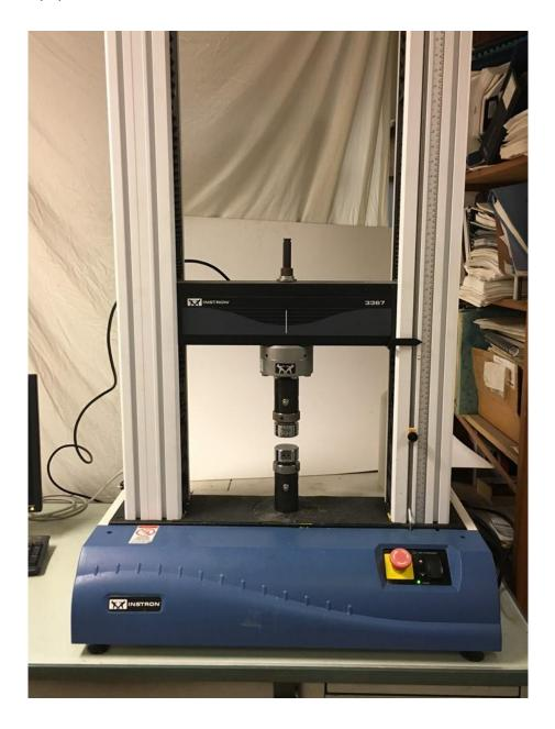
Figure 14 Quasi Static mechanical testing machine (Instron Model 3367).
