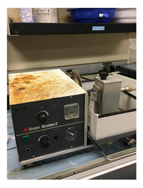
Figure 18 Struers Accutom-2 was used as the cutting machine.
