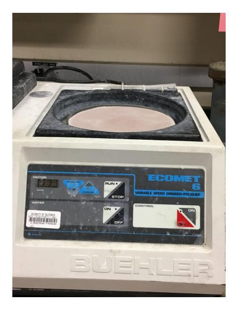
Figure 19 Ecomet 6 was used for polishing using the SiC papers and polishing cloth.
