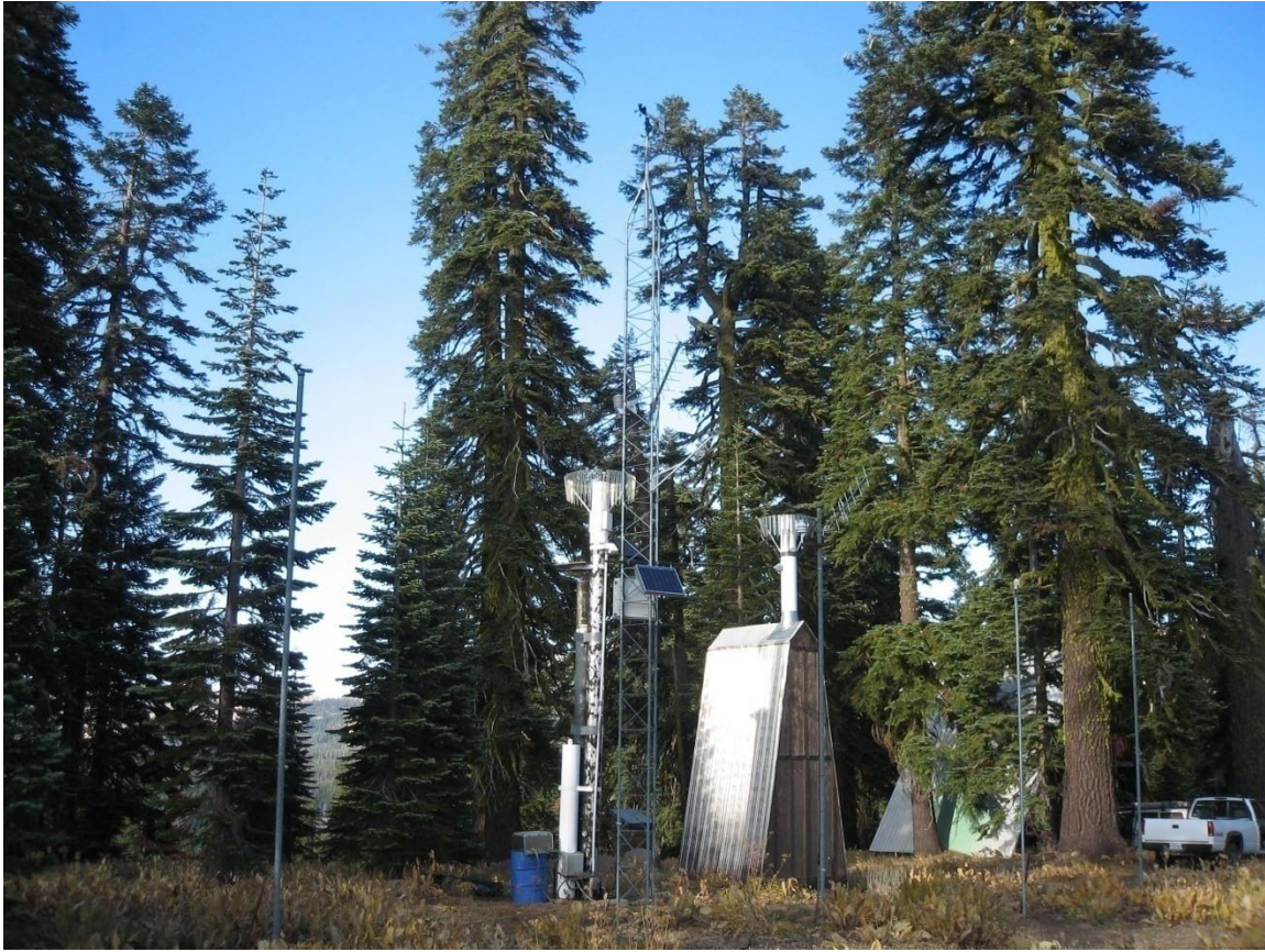
Figure 25. Alpha station, elevation 2334 m / 7657 ft. Site has provided snow measurements for California Department of Water Resources for many years . New tower latticework with anemometer is visible just to right of leftmost white precipitation gauge.
