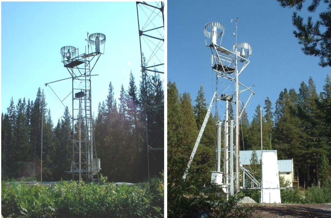
Figure 17. Central Sierra Snow Lab. Left: View to south. Geonor gage left, Belfort gage right, anemometer above both, snow depth sensor to left. Tower is 8 m / 25 ft high. Right: View to north, tower, snow protection shelter, caretaker residence in back.
