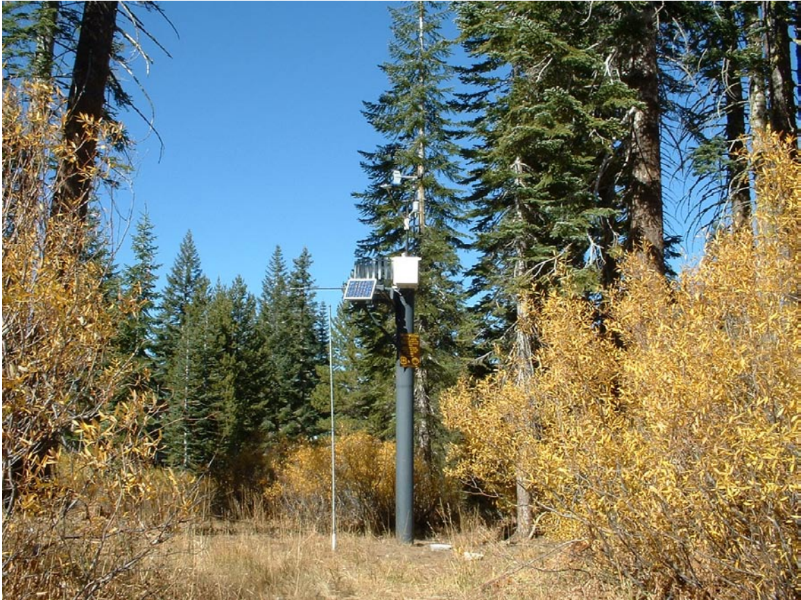
Figure 21. Sugar Bowl lower site (2126 m / 6975 ft). View is approximately to northwest. Site has AC power and heated tipping bucket precipitation gauge. Photo by Dave Simeral.
