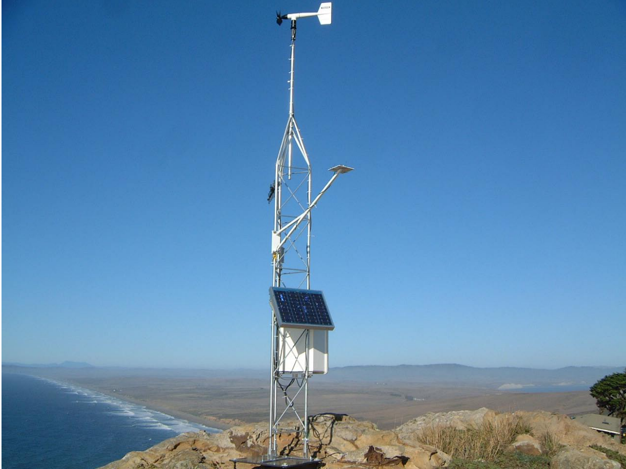
Figure 5. Point Reyes Lighthouse Rock climate station, 160 m (526 ft) above Pacific Ocean. Looking toward north. For orientation, solar panels always point due south. Point Reyes RCA building and climate station is approximately 11 km (7 mi) distant behind the tower and just below the protective enclosure.
