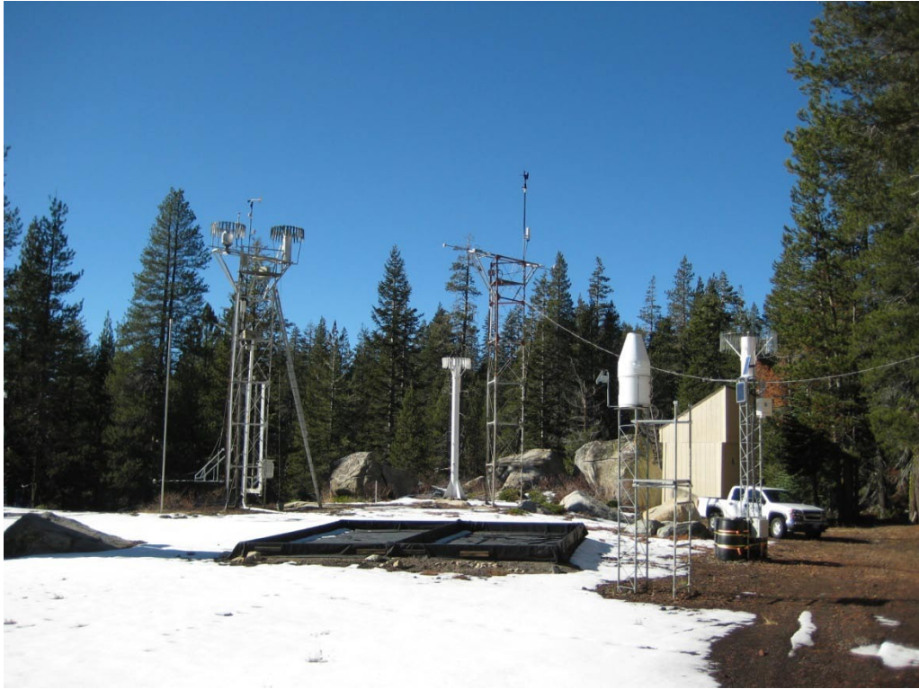
Figure 18. Research equipment at Central Sierra Snow Lab. ECCM equipment on left tower. NRCS Snotel precipitation gauge (white) in center.
