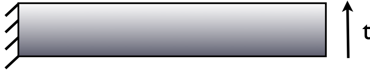
Figure 8.7: Figure of a beam under transverse shear loading conditions. The fibers are assumed to go along the length of the beam.
