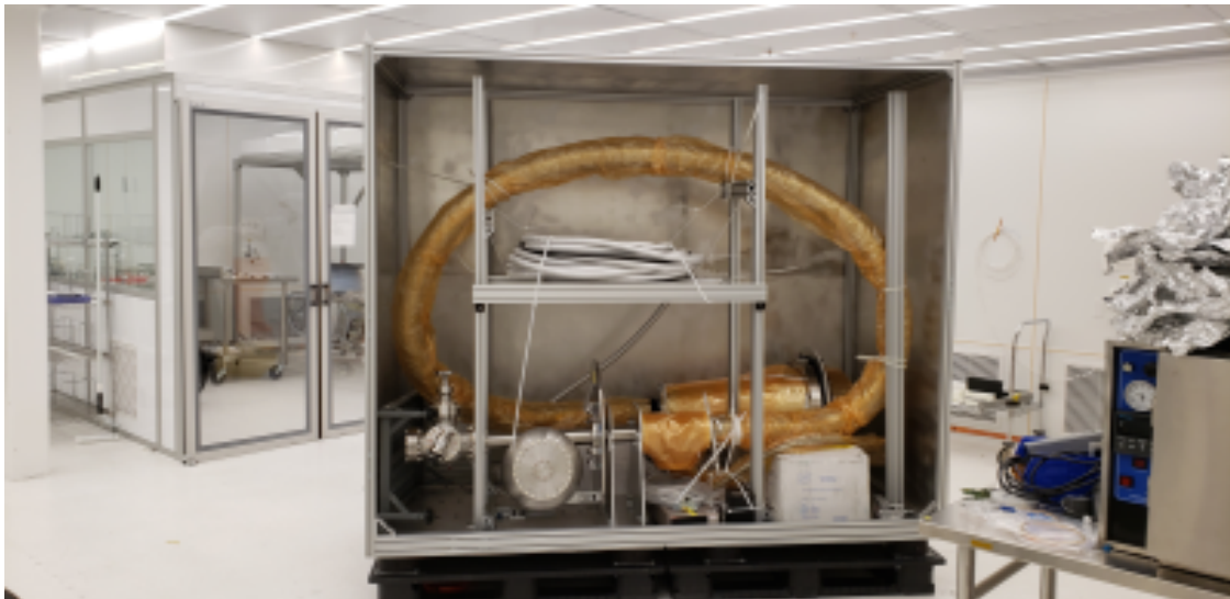
Figure 3.40: A photograph of the cathode high voltage delivery crate. Aluminum panels lined the box. The plastic wrap kept the bellows relatively dust free, despite the box not being airtight. Assorted tools necessary for installation were shipped in the same box. The HV cable is seen spooled on the top, protected by a separate plastic sheath. A challenge of this method was orienting the bellows correctly to minimize strain and torsion.
