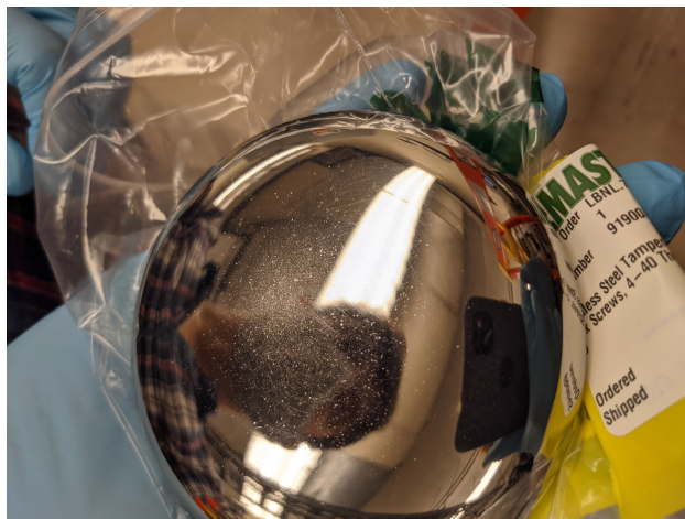
Figure 8.32: The XeBrA electrodes after hundreds of breakdowns, showing damage in the form of white pits.
