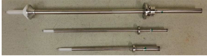
Figure 3.2: Photographs of examples of traditional feedthrough designs for dual-phase TPCs. From top to bottom: the designs for DUNE far-detector, Darkside, and CAPTAIN TPCs. Photograph taken from [102].
