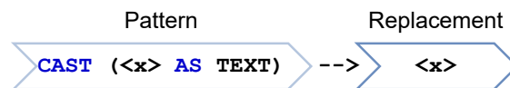
Figure 4.4: Alice formulates a rule to remove CAST(... AS TEXT) expressions using the VarSQL language [88]. In VarSQL’s syntax, <x> is an element-variable that represents a table, column, value, expression, predicate, or sub-query.
