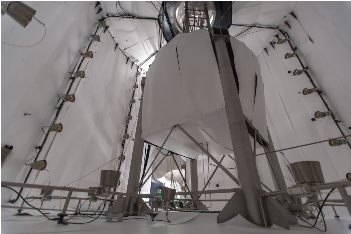
Figure 2.7: View of the inside of the WCD. The stainless steel sphere of the LSV is shrouded in Tyvek reflector at the center. PMTs are mounted on the wall and floor of the WCD.
