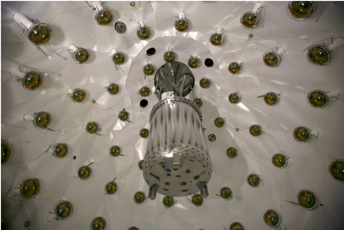
Figure 2.6: View of the inside of the LSV. The metal can in the center is the TPC cryostat. The PMTs and Lumirror reflectors line the wall.
