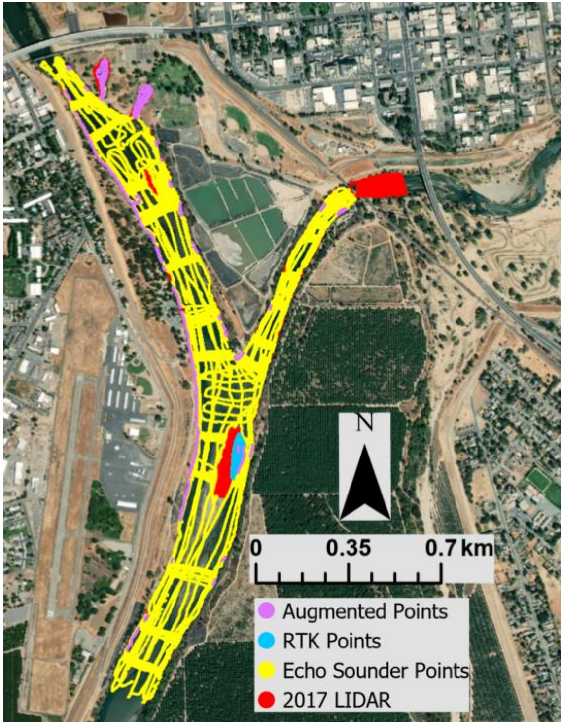
Figure A.A.7. Sources of elevation point data used to construct the final digital elevation model used in this study.
