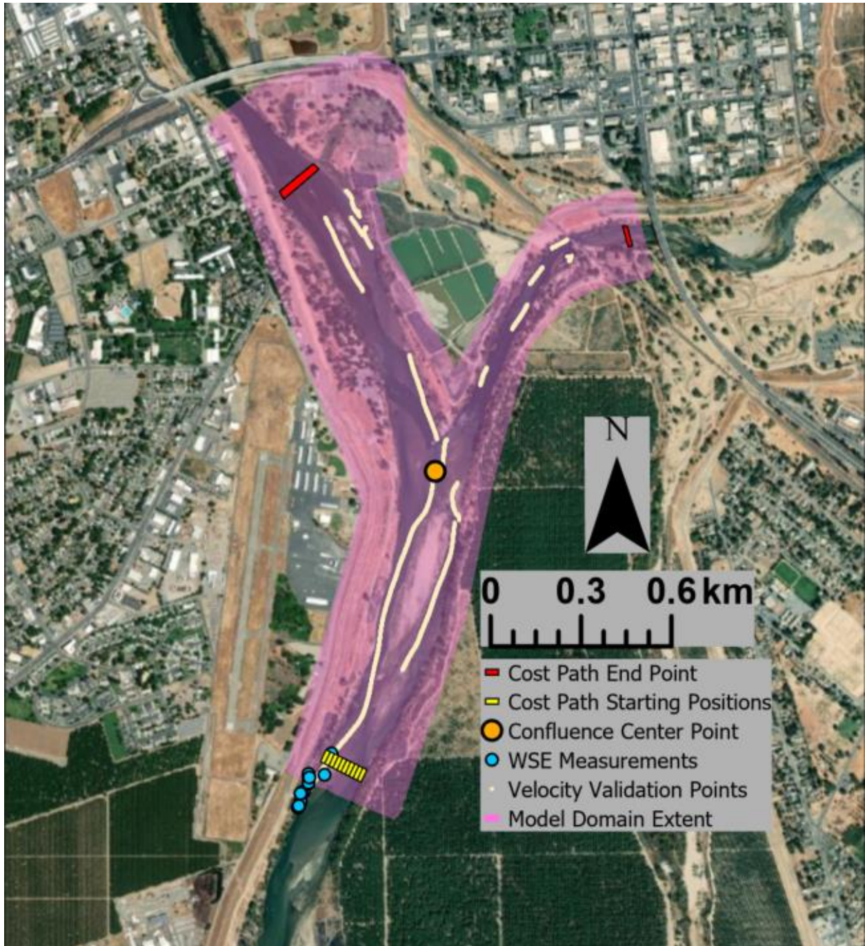
Figure 2.3. Map of the study area including the extent of the model domain, start and end points for the cost path analysis, kayak validation survey transects, and water surface elevation survey locations.
