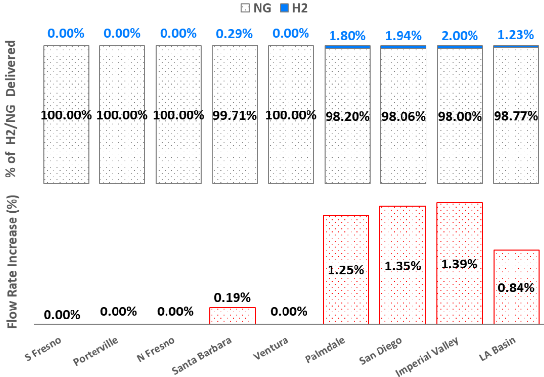
Figure 5.31. Hydrogen to natural gas percentage (top) and percent increase of flow rate (bottom) at the demand nodes – scenario 4
