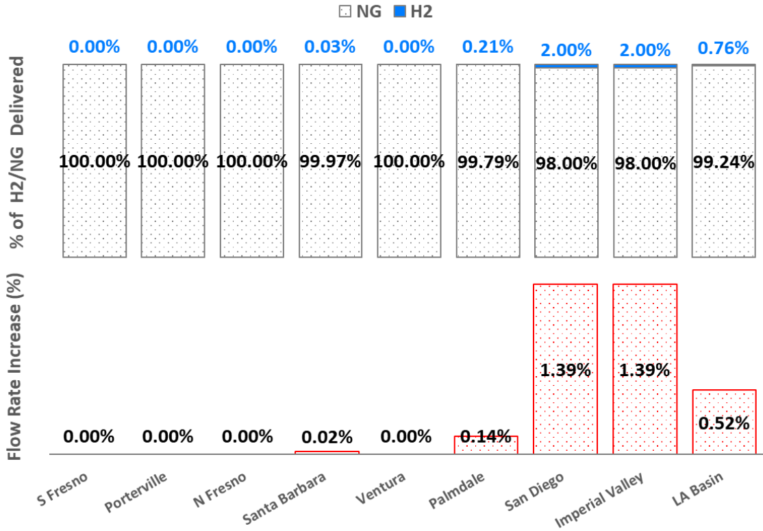
Figure 5.25. Hydrogen to natural gas percentage (top) and percent increase of flow rate (bottom) at the demand nodes – scenario 2
