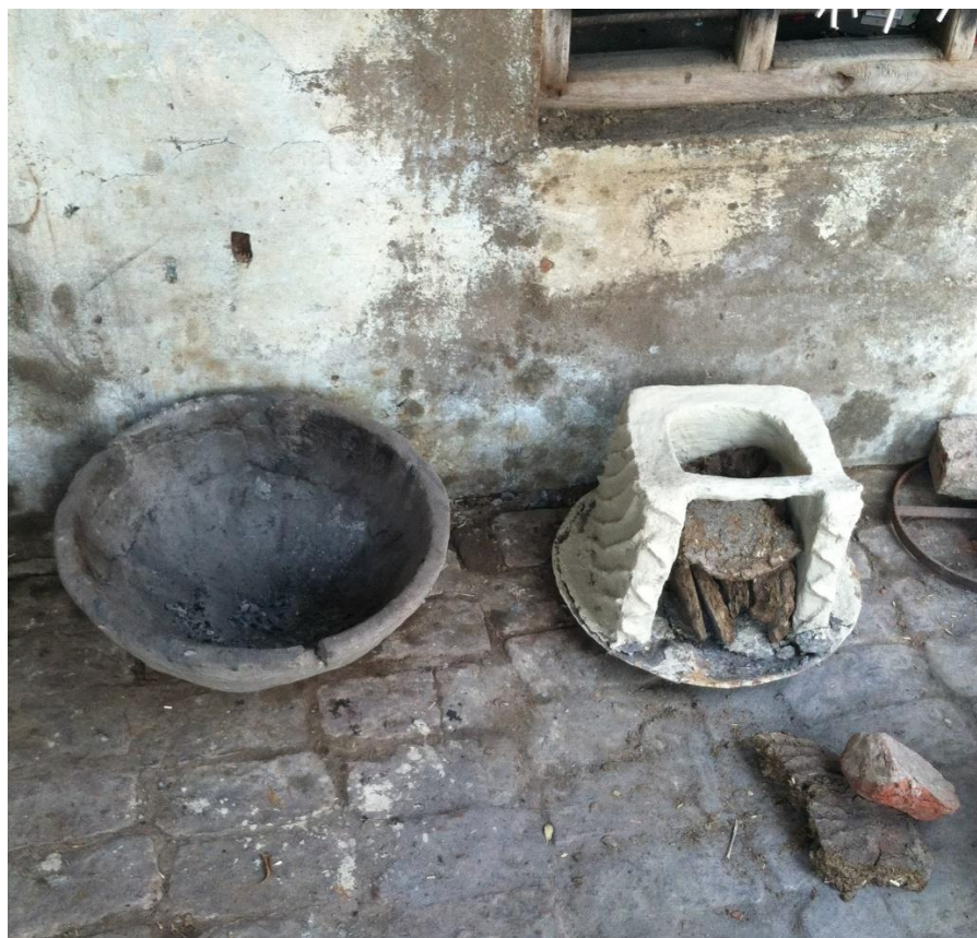
Figure 2: Photograph of traditional mud cookstoves used in India. An angithi stove is pictured on the left and a chulha stove loaded with dung cakes is pictured on the right.
