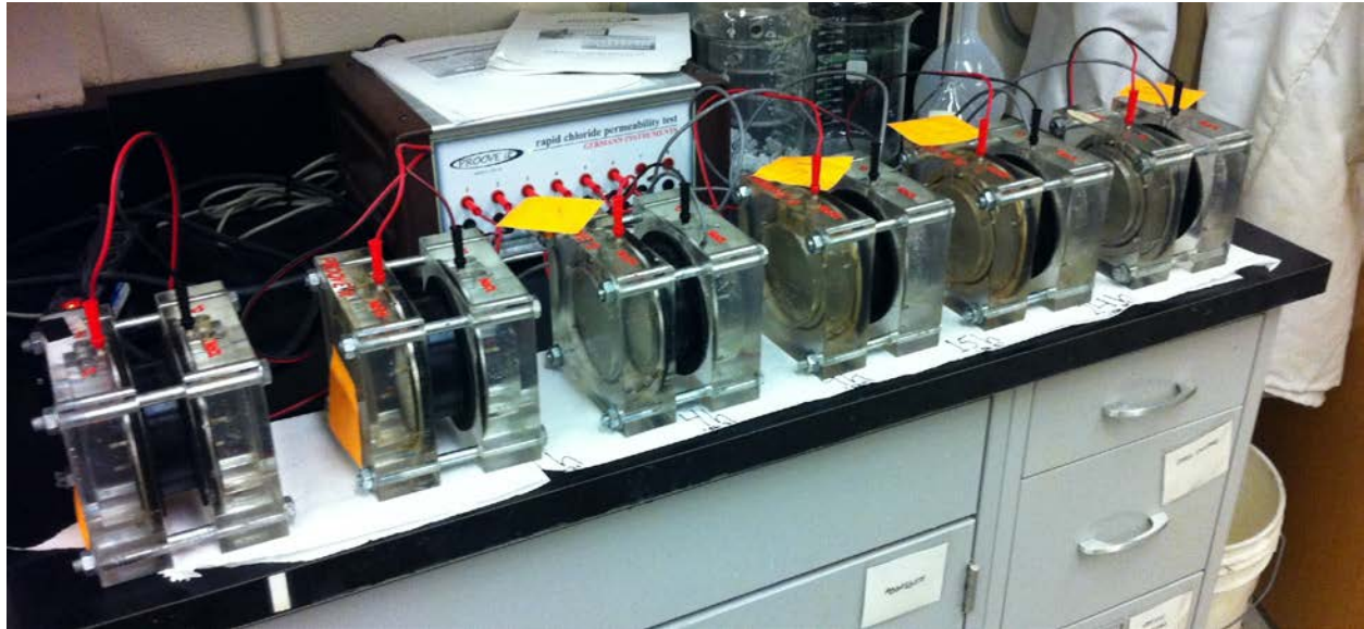
Figure 3-7 NT Build 492 Rapid Testing of Chloride Migration
